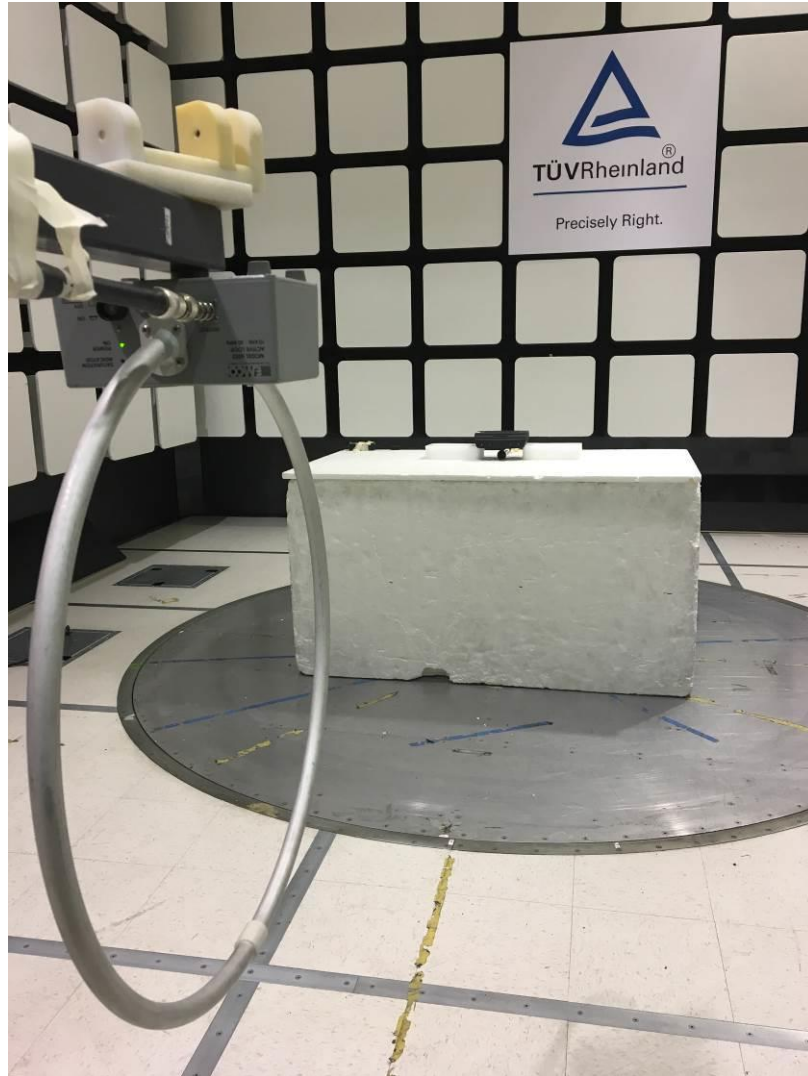
Figure 1: Test Setup for Radiated Emissions 9 kHz to 30 MHz - Front
