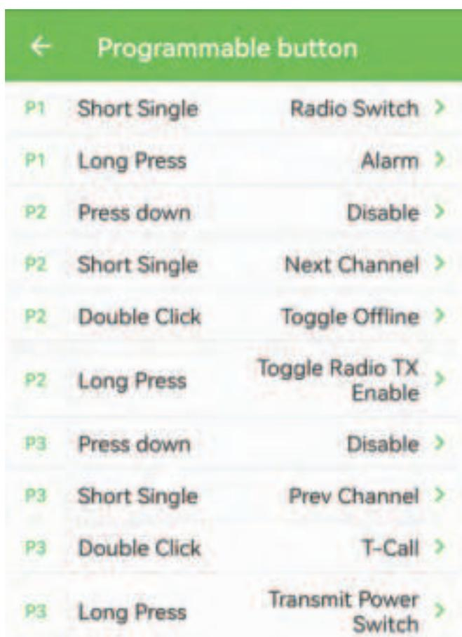
The programming button can define the shortcut operation of P1-P3 button, among them, T-CALL is 1750HZ, Radio Switch is turn on/off FM radio.
