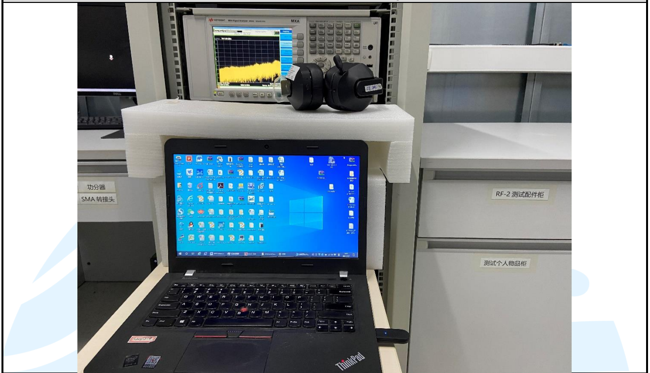
Conducted RF Test Setup
