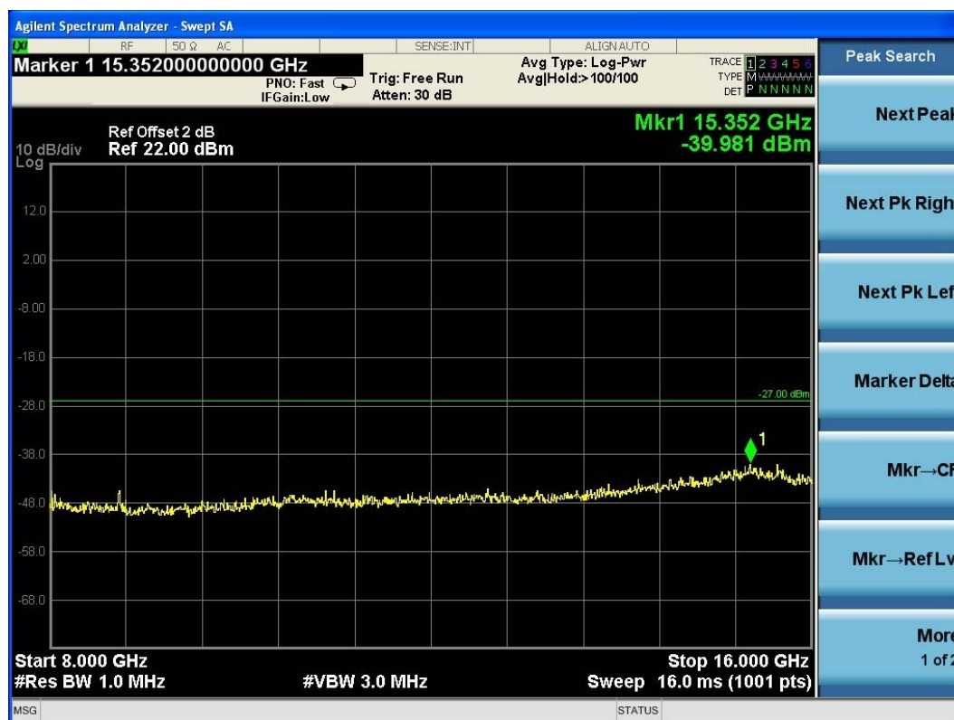
(Plot 4.9.2 C5: Channel 48: 5240MHz @ 802.11n HT20)
