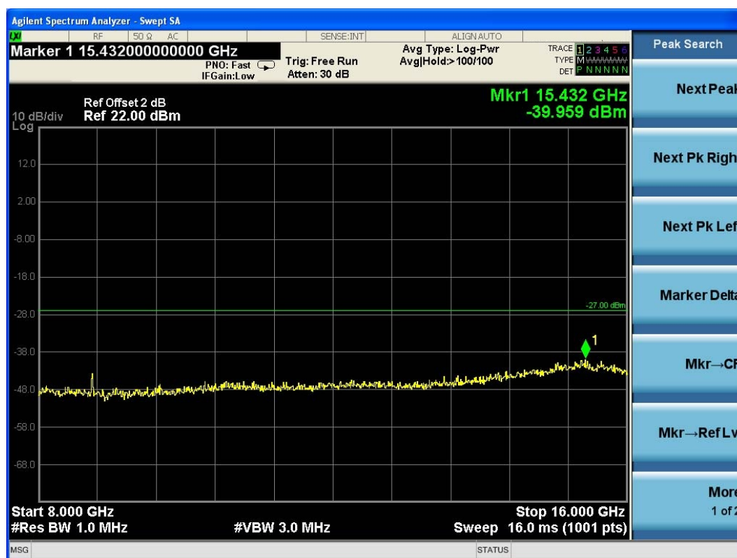
(Plot 4.9.1 C5: Channel 48: 5240MHz @ 802.11a)
