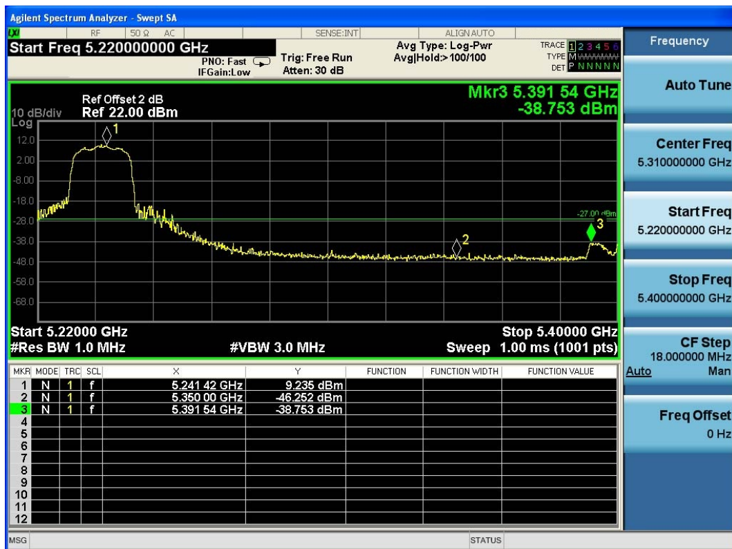
(Plot 4.9.2 C1: Channel 48: 5240MHz @ 802.11n HT20)
