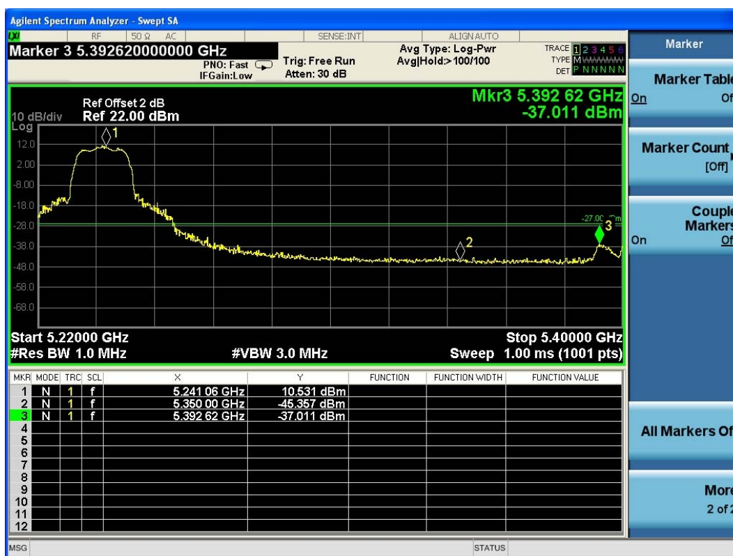
(Plot 4.9.1 C1: Channel 48: 5240MHz @ 802.11a)
