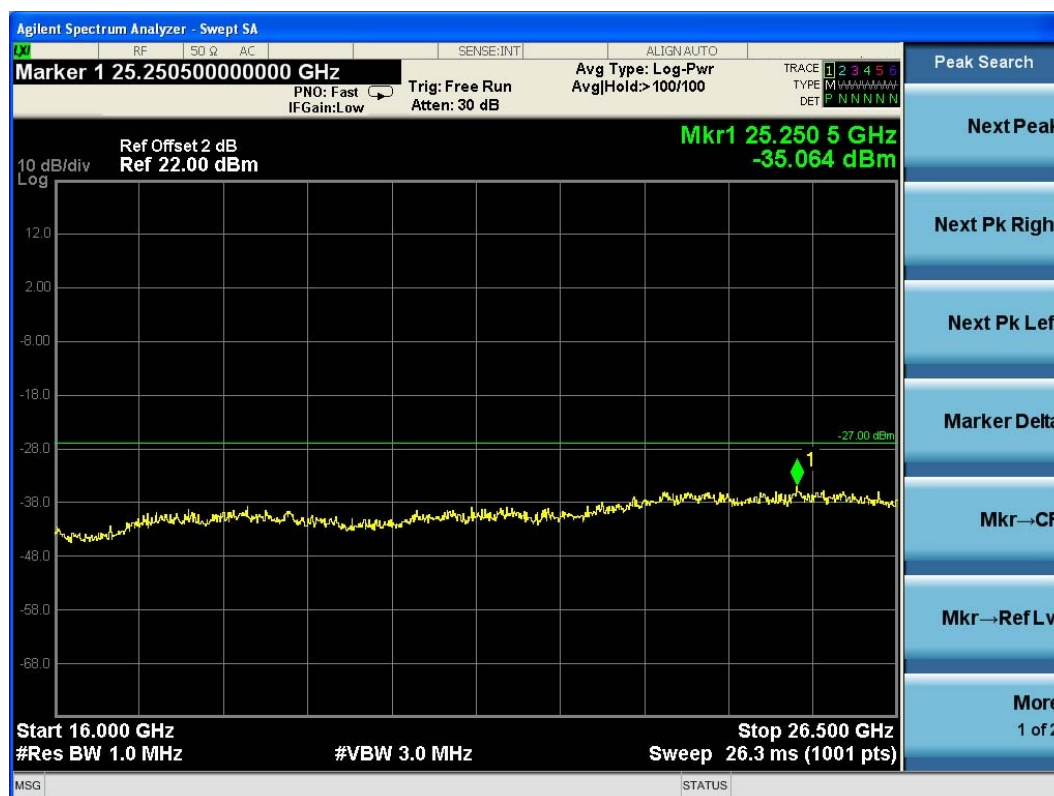
(Plot 4.9.1 A6: Channel 36: 5180MHz @ 802.11a)
