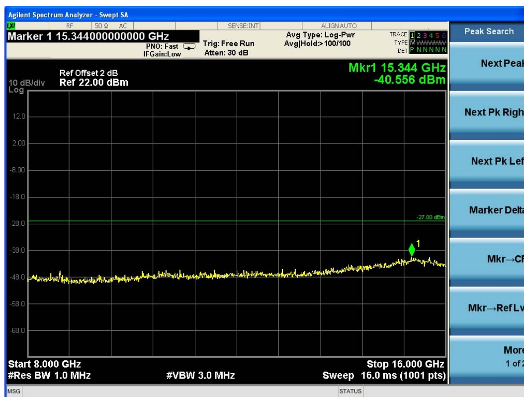
(Plot 4.9.1 A5: Channel 36: 5180MHz @ 802.11a)
