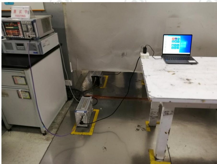
Conducted Emissions Test Setup
