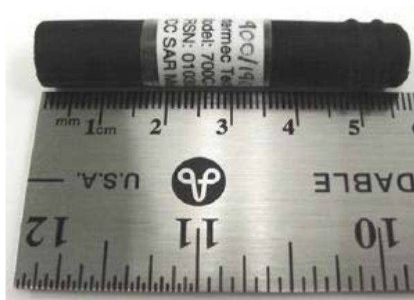
Dual-Band Stubby Antenna (P/N: 805-606-002)
