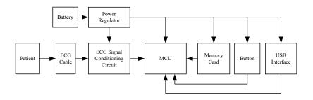
**Electrical Principle Block Diagram of the Recorder**
