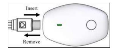
Insert / Remove ECG cable
