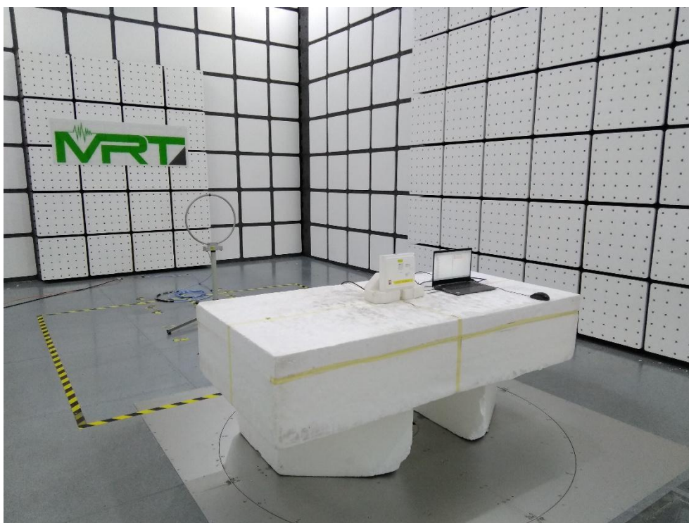
Description: Radiated Emission Test Setup for 9kHz~30MHz
