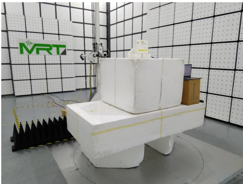
Description: Radiated Emission Test Setup for 9kHz~30MHz
