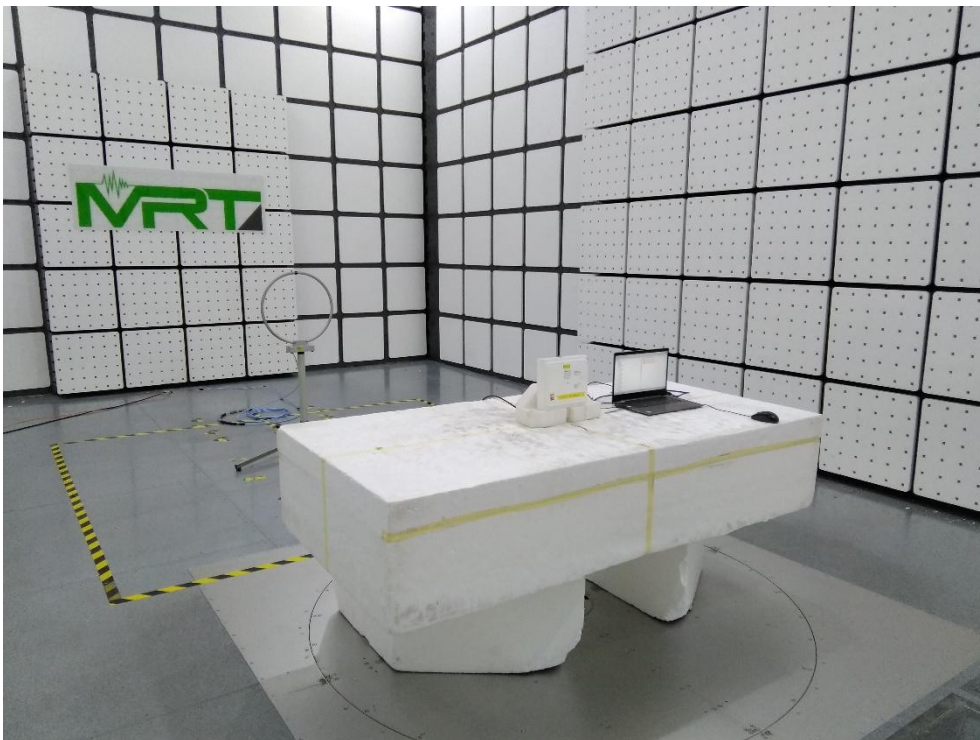
Description: Radiated Emission Test Setup for 9kHz~30MHz
