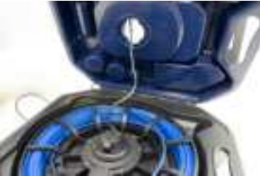
Fig. 60: Wrong: Camera cable not pulled tight
