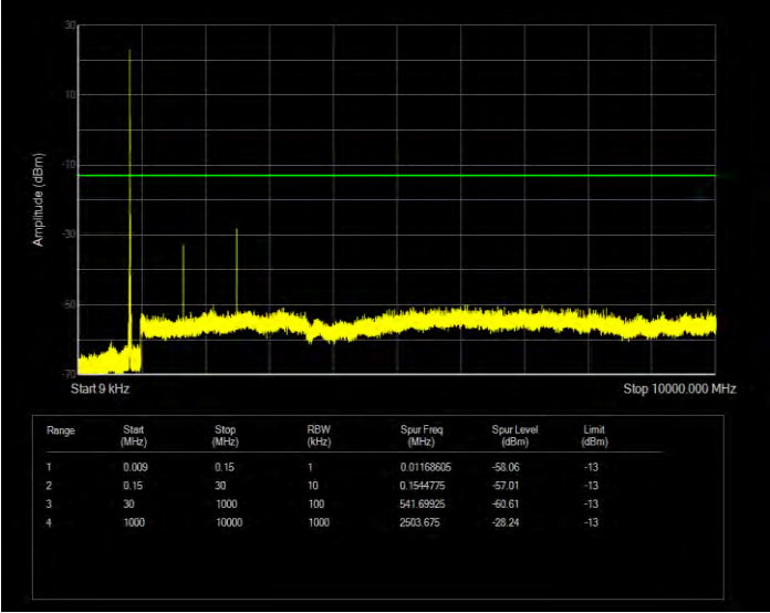
Band26(824-849) 16QAM BW=5MHz Channel=26915 RB Size=1 Position=#0
