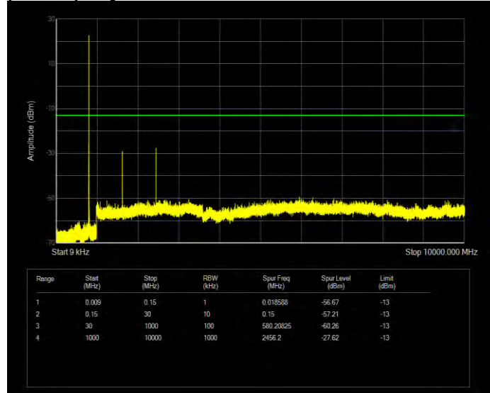
Band26(814-824) 16QAM BW=1.4MHz Channel=26783 RB Size=1 Position=#0
