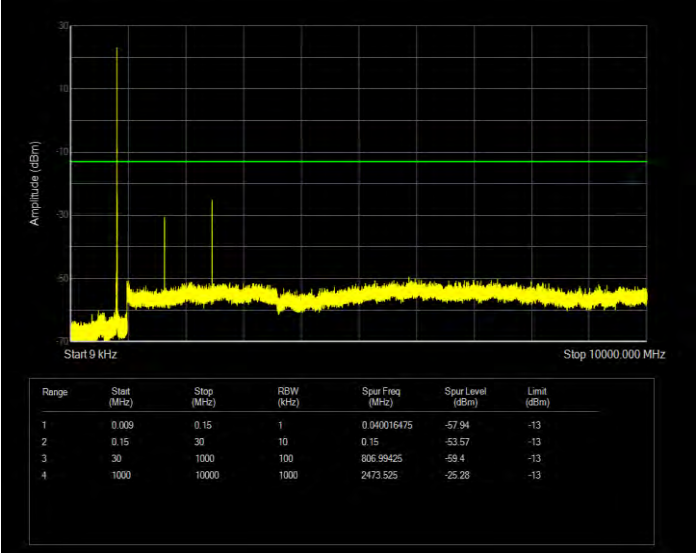
Band26(824-849) QPSK BW=3MHz Channel=26915 RB Size=1 Position=#0
