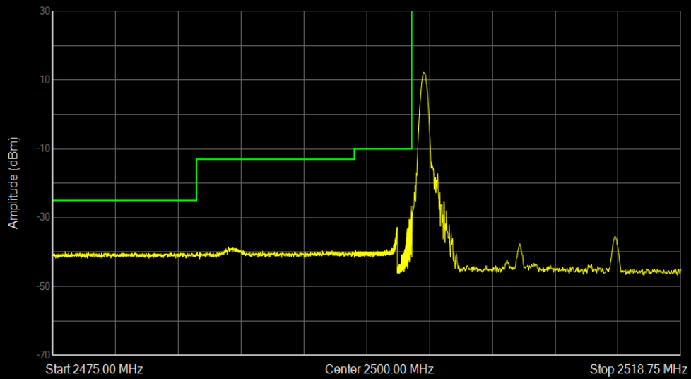
Band7 QPSK BW=15MHz Channel=20825 RB Size=1 Position=#0
