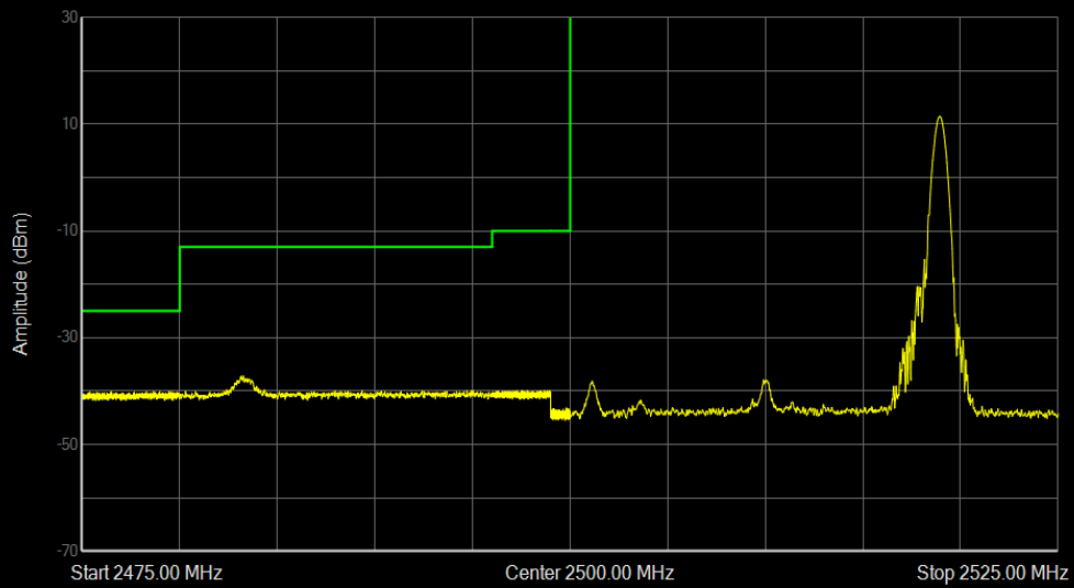
Band7 16QAM BW=20MHz Channel=20850 RB Size=1 Position=#Max
