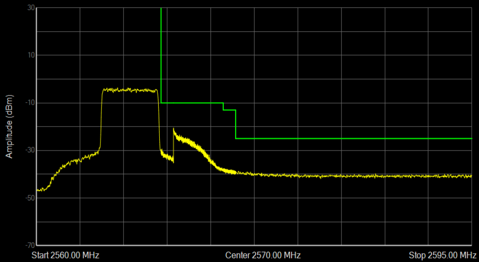
Band7 QPSK BW=5MHz Channel=21425 RB Size=25 Position=#0
