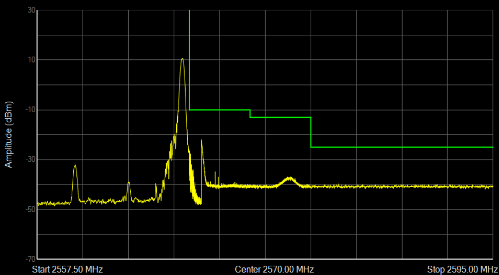
Band7 16QAM BW=10MHz Channel=21400 RB Size=1 Position=#Max
