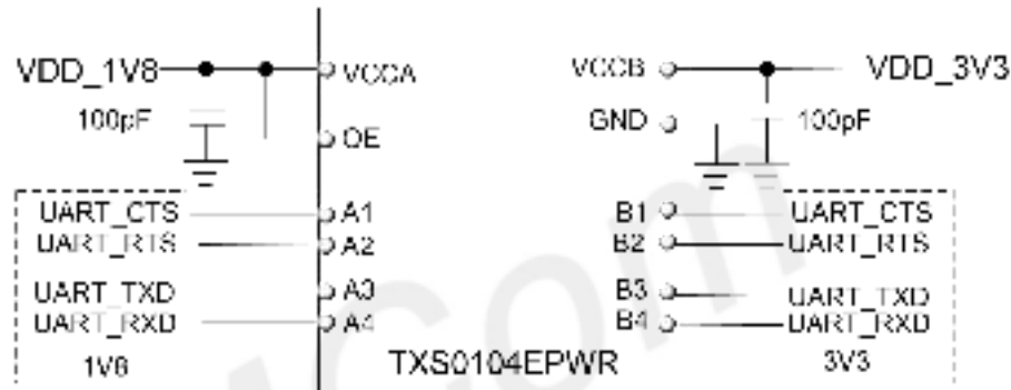
Figure 33: UART level conversion circuit
