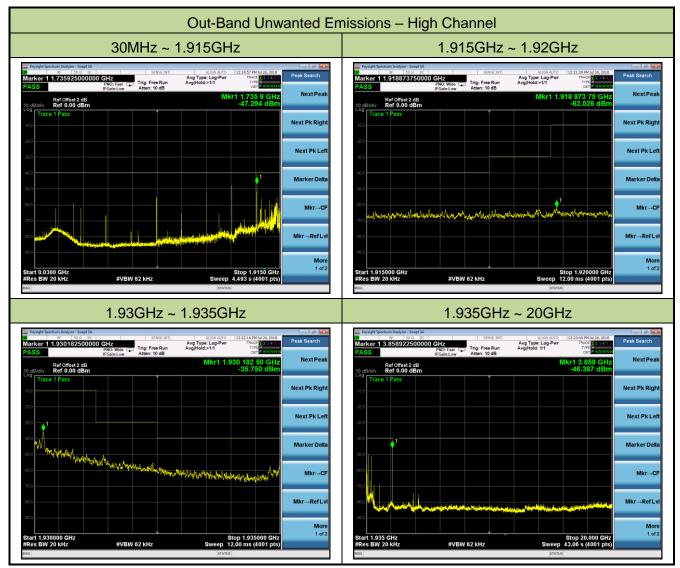
Note 1: The BS spurious out-of-band transmission level is below the indicated limit.
