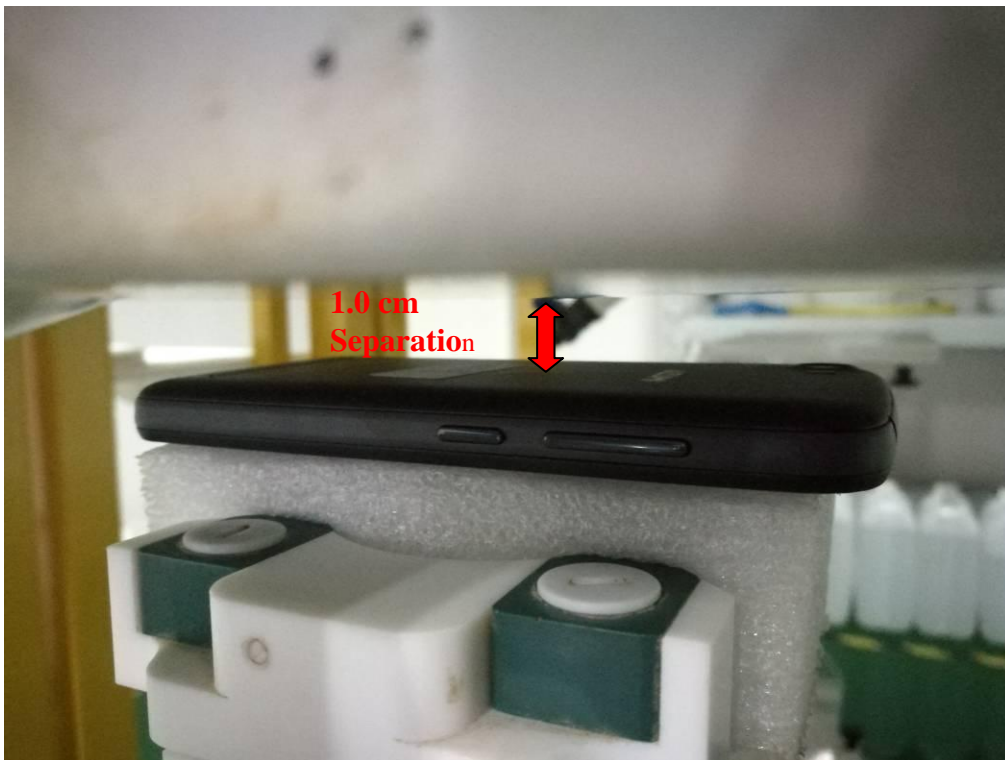
Body Setup Photo (LCD DOWN)
