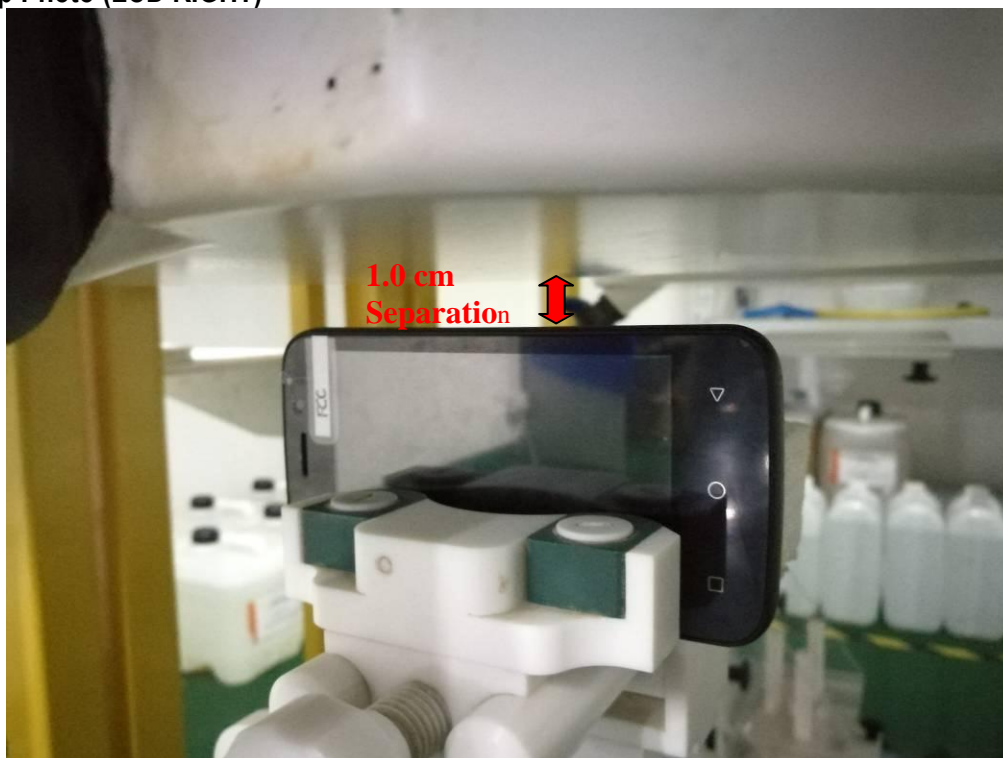
Body Setup Photo (LCD RIGHT)
