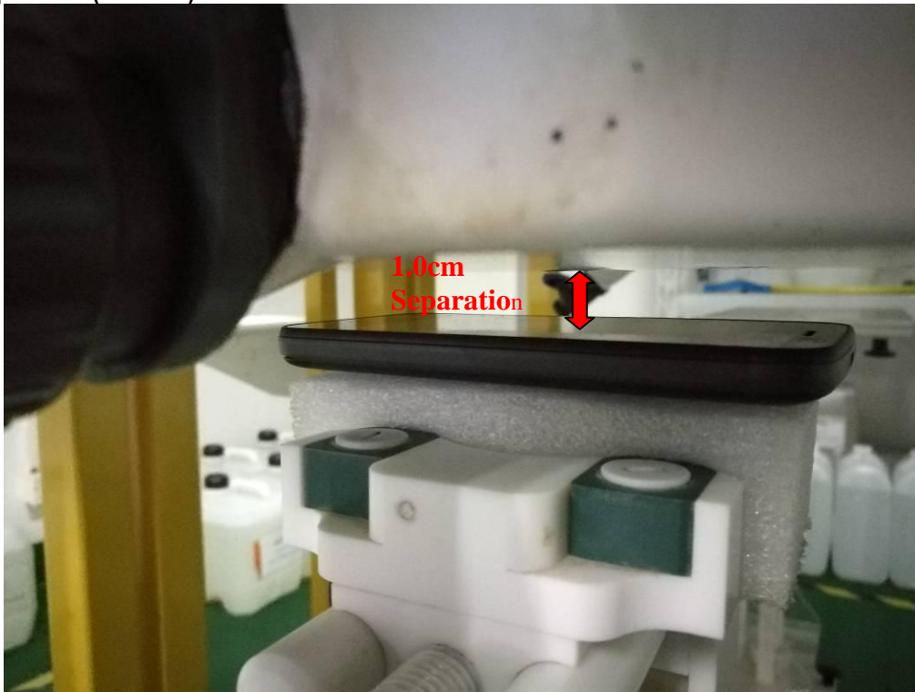
Body Setup Photo (LCD DOWN)
