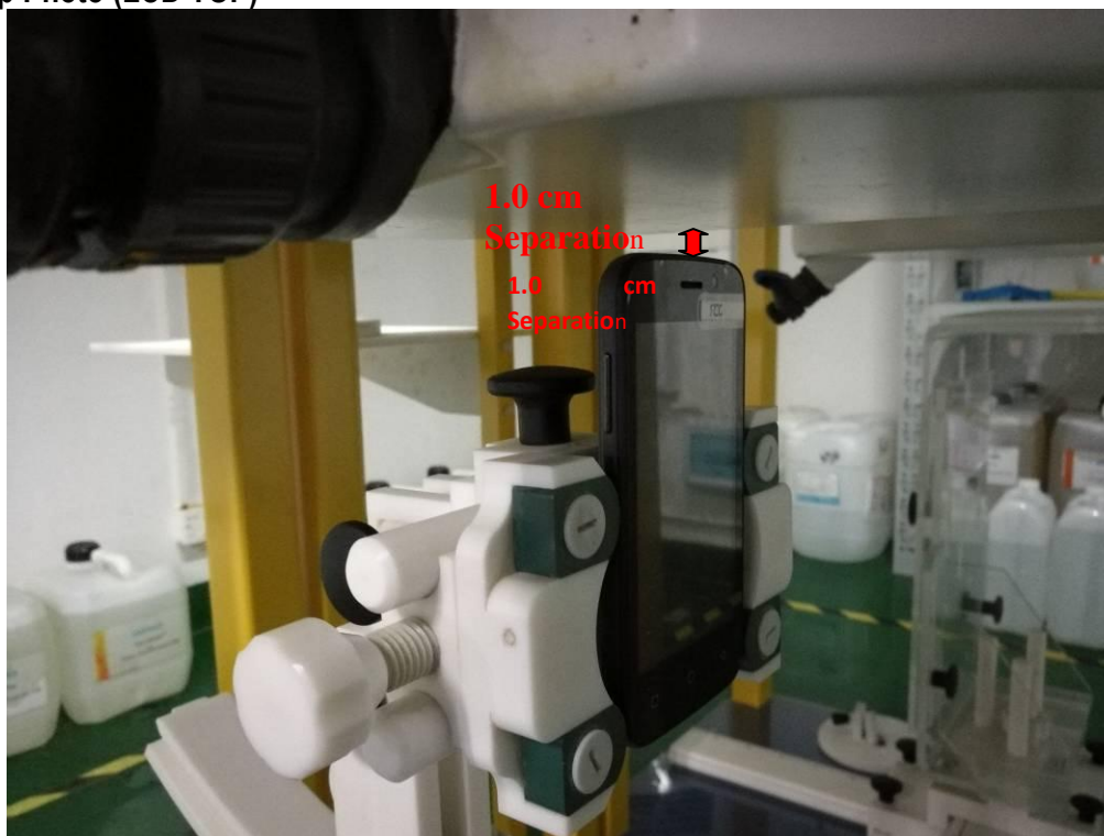
Body Setup Photo (LCD TOP)
