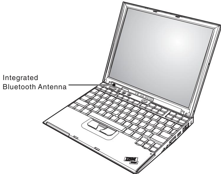
**Note:** The antenna of IBM Integrated *Bluetooth* III with 56K Modem is located on the bottom of the computer lid. Transmitted energy from the *Bluetooth* device is very low compared to other RF devices. Therefore a 20 cm separation from the *Bluetooth* antenna is not required.
