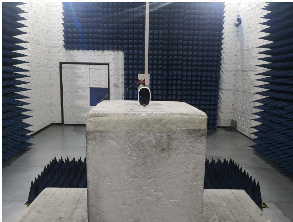
FCC RADIATED EMISSION TEST SETUP ABOVE 1GHZ
