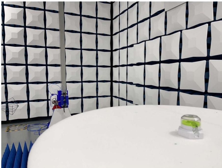
Set-up for Radiated Emission (1GHz above)
