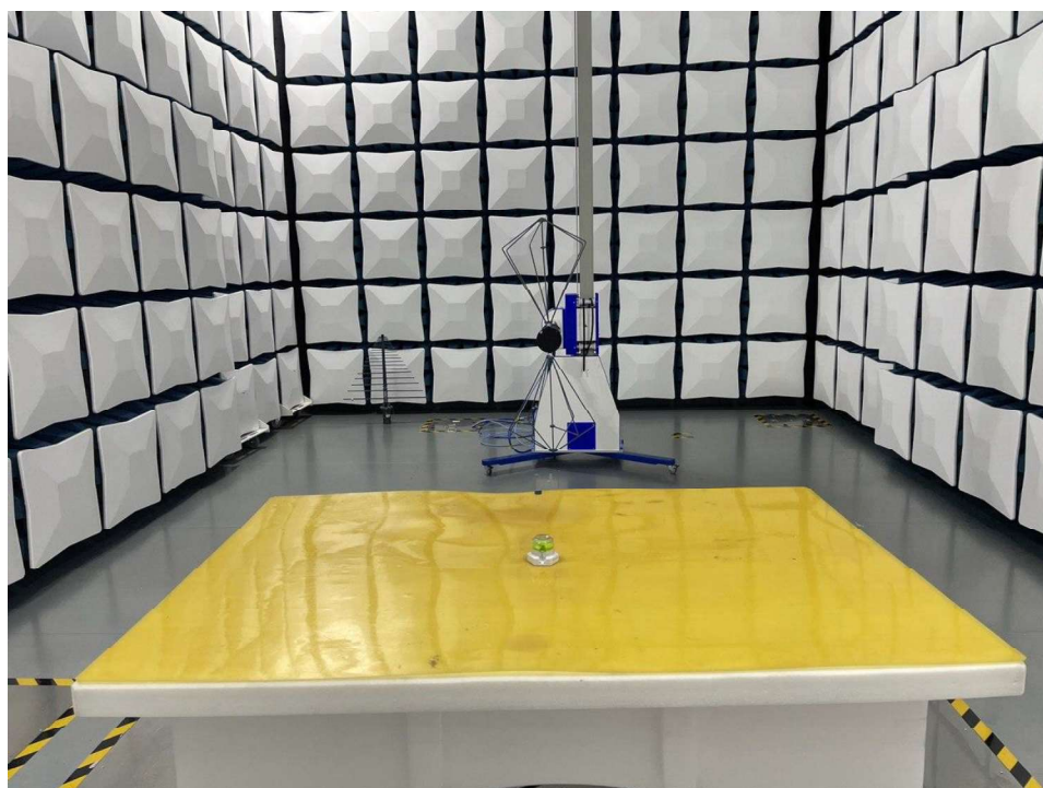
Set-up for Radiated Emission (30-200MHz)
