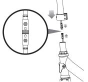
2 Join the connectors from the T-bar to the fork. Loosen the collar clamp on the T-bar with a side-toside twisting motion, install the T-bar to the fork until it bottoms out on the headset locknut.
