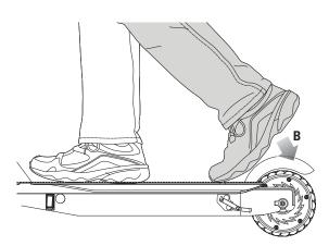
**Note:** As an additional safety feature, the scooter is designed to cut power to the motor when the brake is applied.
