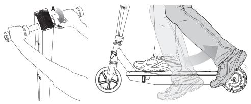
Note: Scooter must accelerate to at least 3 mph (5 km/h) for motor to engage.
