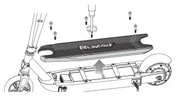
**1** Using a Phillips screwdriver, remove the six (6) screws and remove the deck plate.
