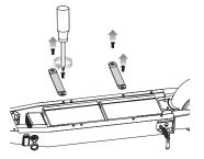
**3** Using a Phillips screwdriver, remove the four (4) screws and remove the battery straps. (Note: These are smaller screws than step 1.)
