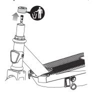
**1** Before inserting the T-bar onto the fork, carefully pull the connector through the rubber protector to remove. Discard the rubber protector.
