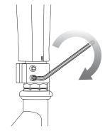
3 With the front wheel pointed straight ahead and the handlebars square to the front wheel, tighten both bolts on the clamp with a 5 mm Allen wrench. Tighten securely.
