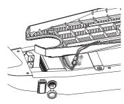
**2** Disconnect the wire from the controller to the deck. Set the deck aside.
