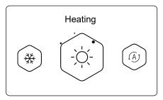
Press ( or ) to change the operation mode. Three modes are optional:, Heating, Cooling, and Auto.
