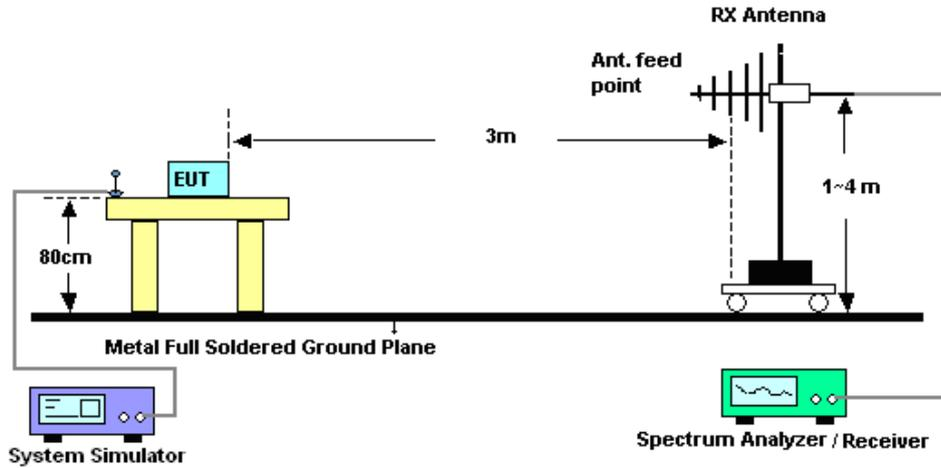
For radiated test above 1GHz
