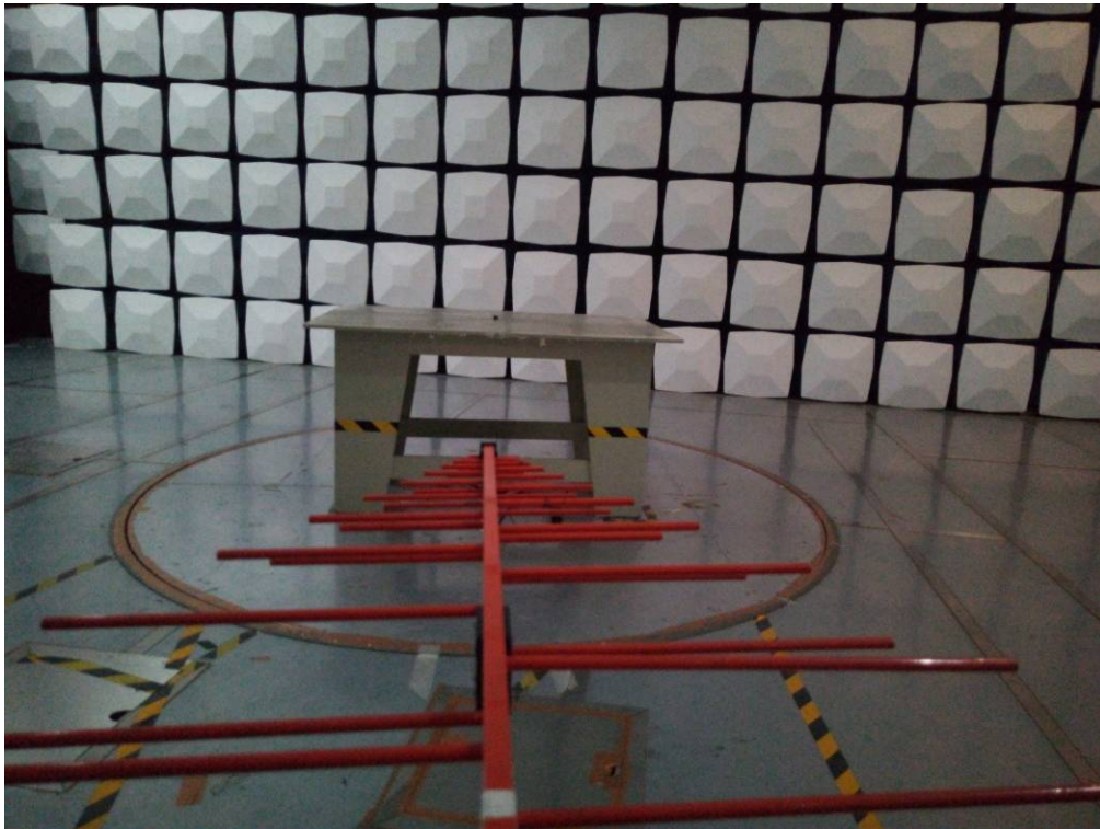
Radiated Emission Below 1GHz View
