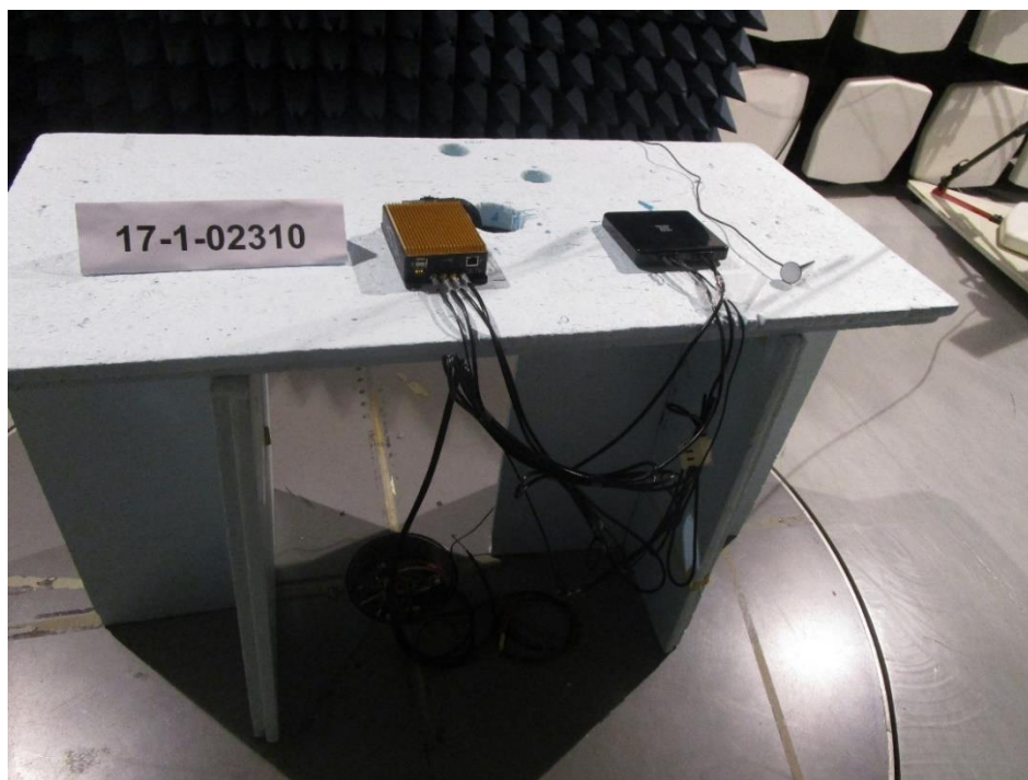
Figure 7: Close View 9 KHz – 30 MHz EUT Laying
