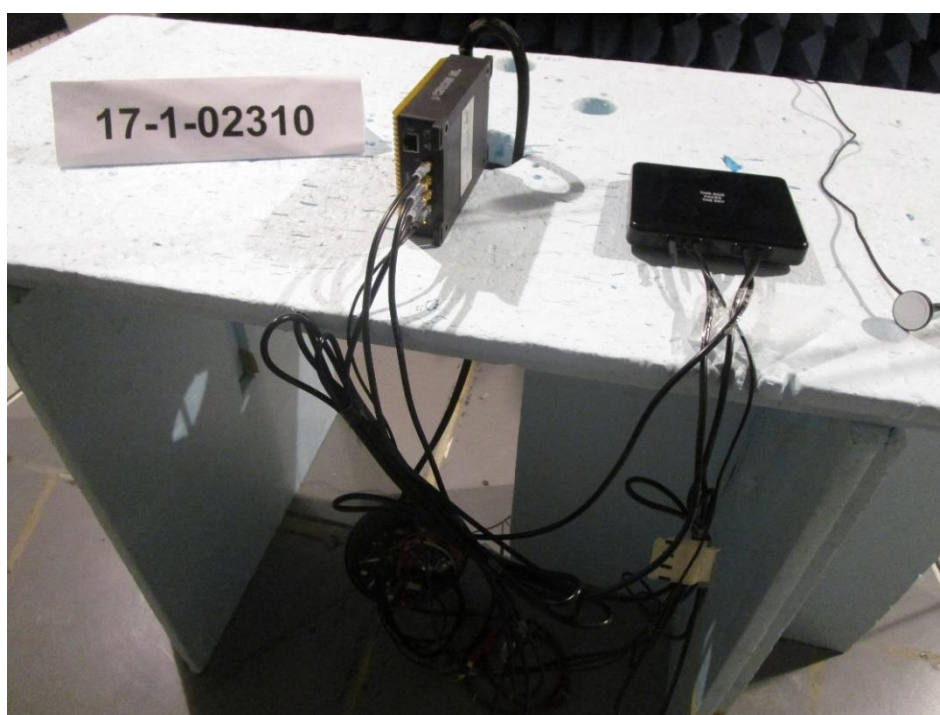
Figure 8: Close View 9 KHz – 30 MHz EUT Standing
