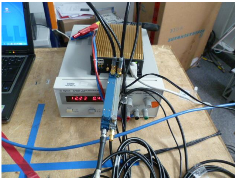
Figure 3: μCROS SL Close View Conducted Sample for WLAN Testing
