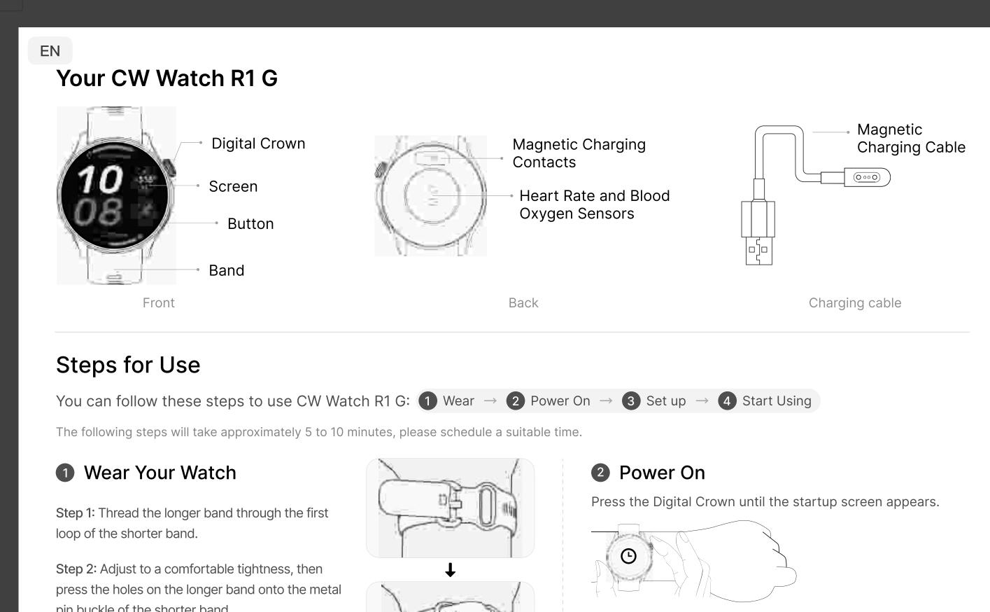
Step 3: Insert the longer band into the second loop
