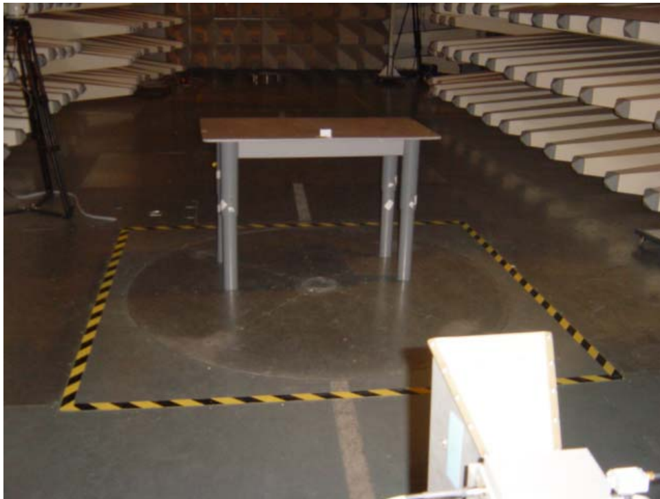
Set-up for Radiation Emission (Transceiver)
