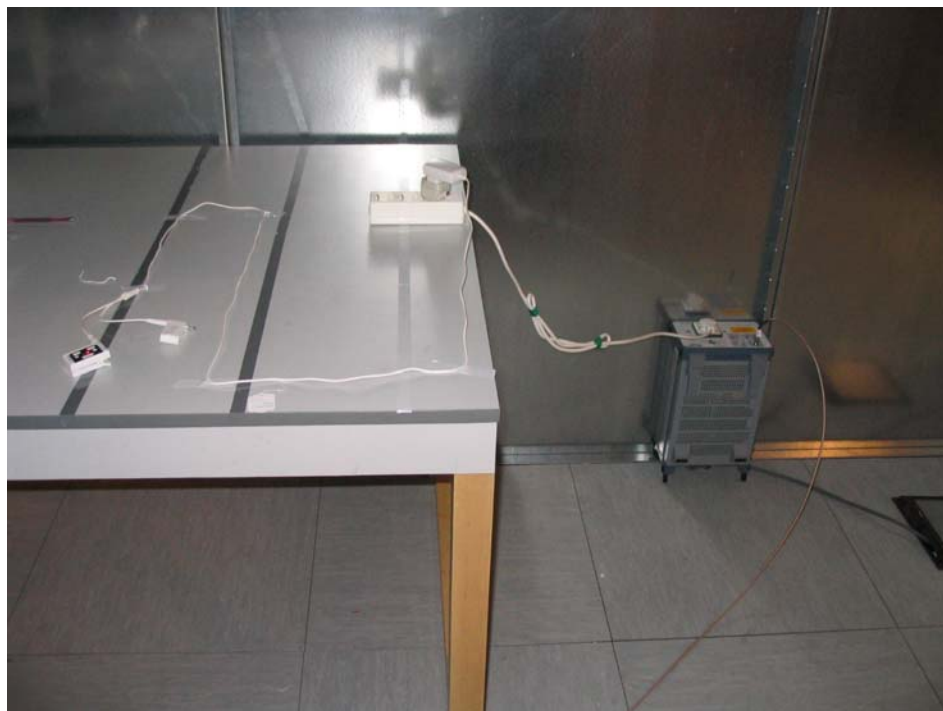
Set-up for Disturbance Voltage on AC mains
