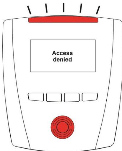
**Figure 5.5** - Information display after reading a data carrier (access denied - red lights)
