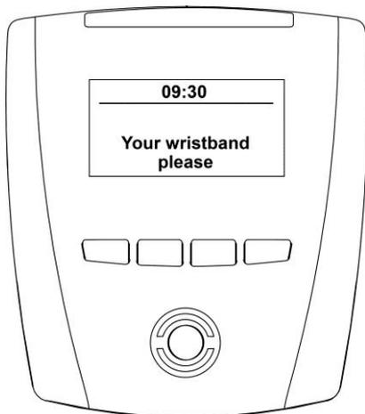
**Figure 5.2** - Start screen of normal function mode of a GAT Access 6100, waiting for data carrier
