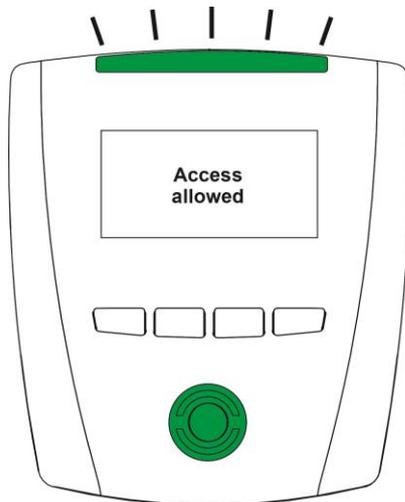
**Figure 5.4** - Information display after reading a data carrier (access granted - green lights)
