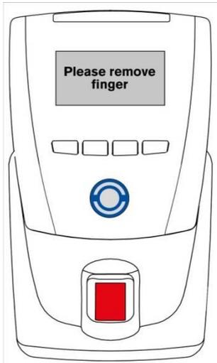
If the fingerprint was scanned correctly, the display shows a message instructing the visitor to remove their finger from the sensor.
