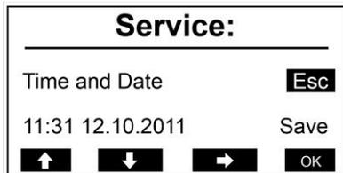
Figure 4.9 - Setting time and date of a GAT Access 6100
