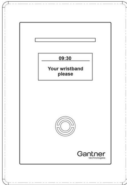
**Figure 5.8** - Information display of GAT TimeAxx 6150 in idle state
