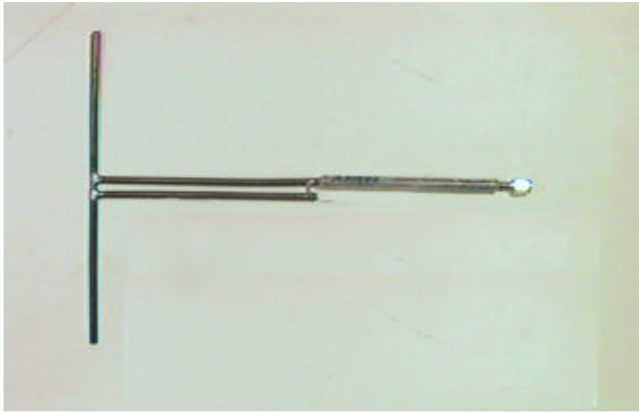
Reference Dipole Antenna Used for ERP Measurement
