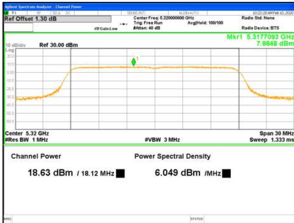
Figure 13: RMS Max Power-5320MHz-802.11ac VHT20-MCS0-TP19-1x2-CH0 (RSS)
