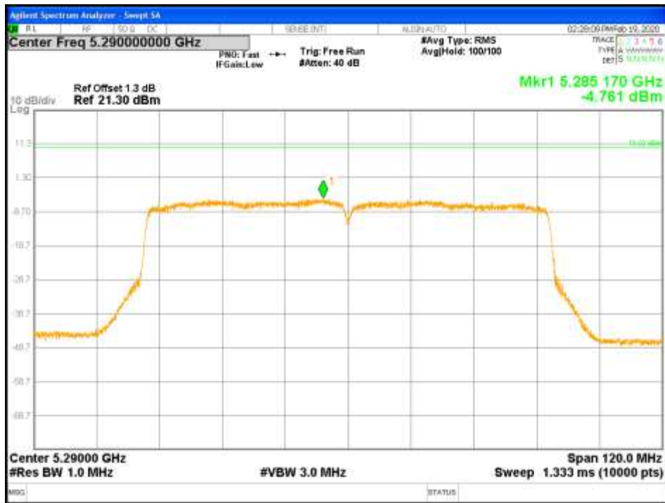
Figure 78: PPSD-5290MHz-802.11ac VHT80-MCS0-TP13-CH1-2x2 (RSS)
