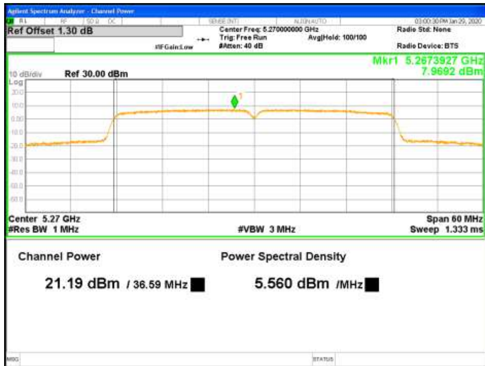
Figure 17: RMS Max Power-5270MHz-802.11ac VHT40-MCS0-TP21-1x2-CH0 (FCC)
