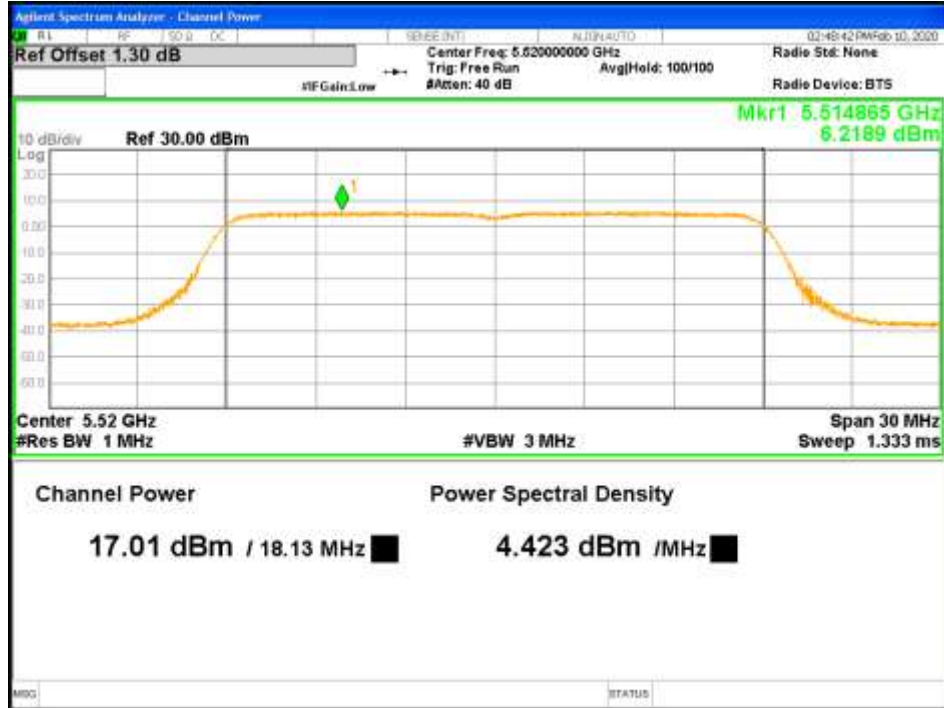
Figure 36: RMS Max Power-5520MHz-802.11ac VHT20-MCS0-TP17-2x2-CH1
