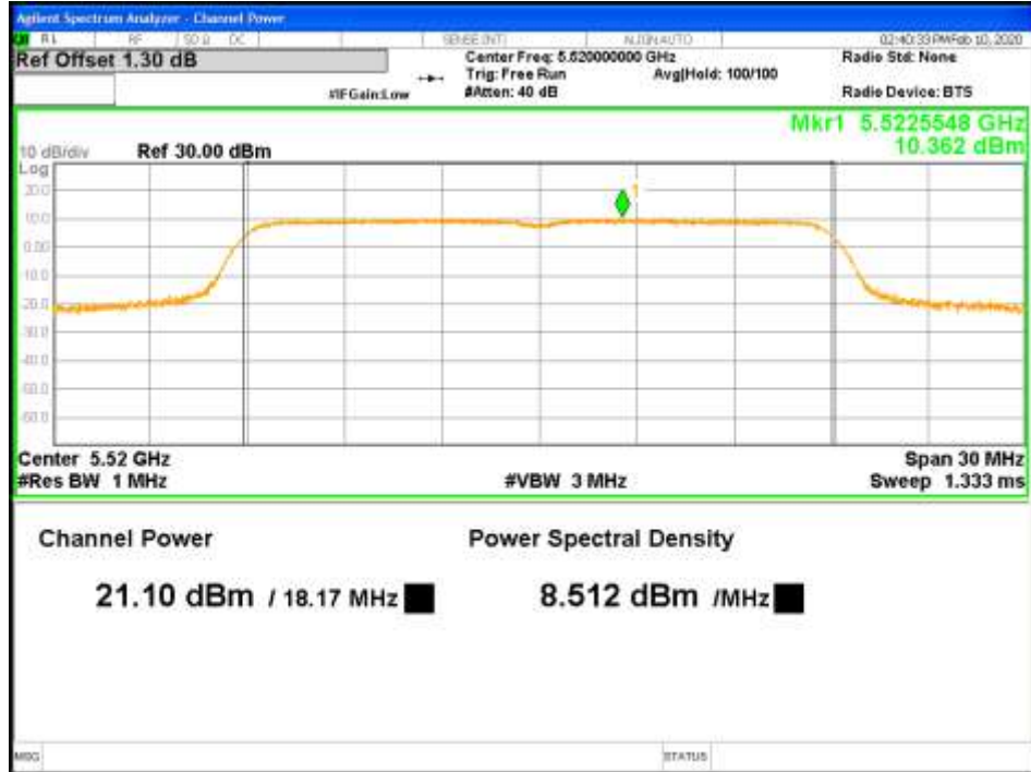
Figure 16: RMS Max Power-5520MHz-802.11ac VHT20-MCS0-TP21-1x2-CH1
