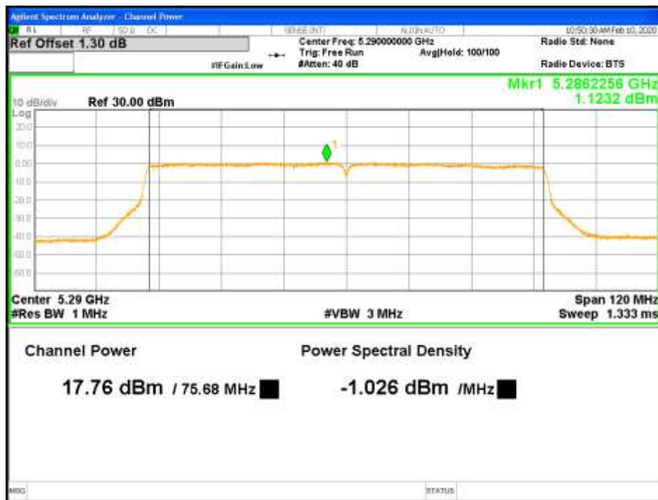
Figure 23: RMS Max Power-5290MHz-802.11ac VHT80-MCS0-TP18.5-1x2-CH0 (FCC & RSS)
