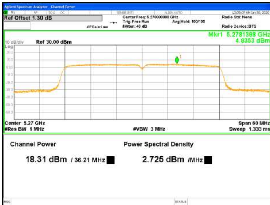
Figure 37: RMS Max Power-5270MHz-802.11ac VHT40-MCS0-TP18.5-2x2-CH0 (FCC)
