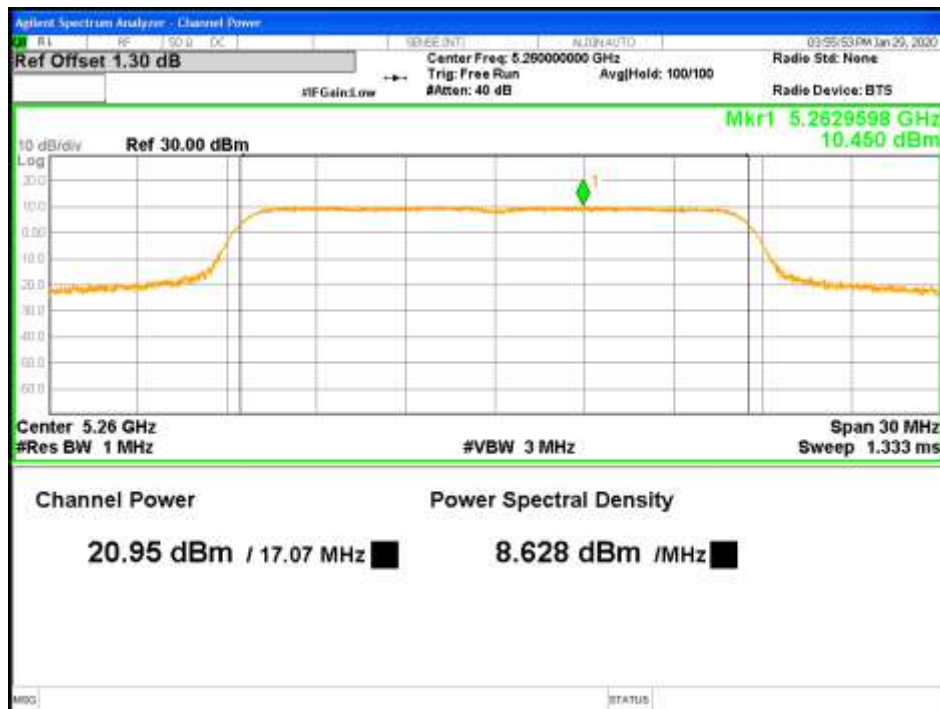
Figure 6: RMS Max Power-5260MHz-802.11a-6Mbps-TP21-1x2-CH1 (FCC)
