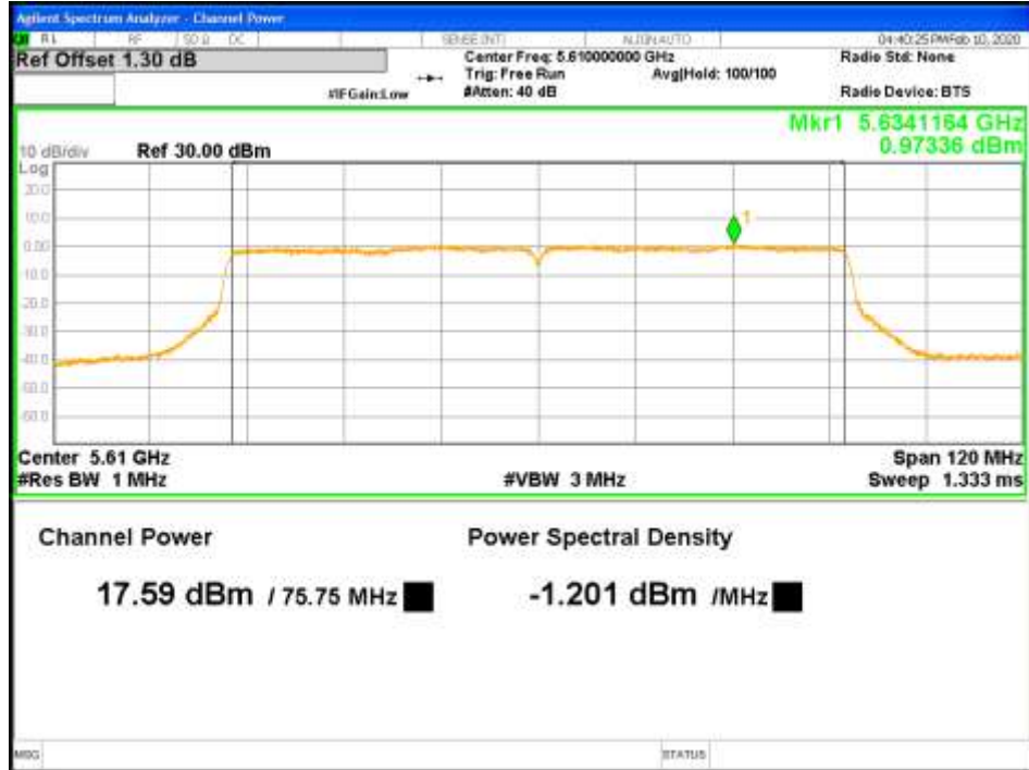
Figure 48: RMS Max Power-5610MHz-802.11ac VHT80-MCS0-TP19-2x2-CH1
