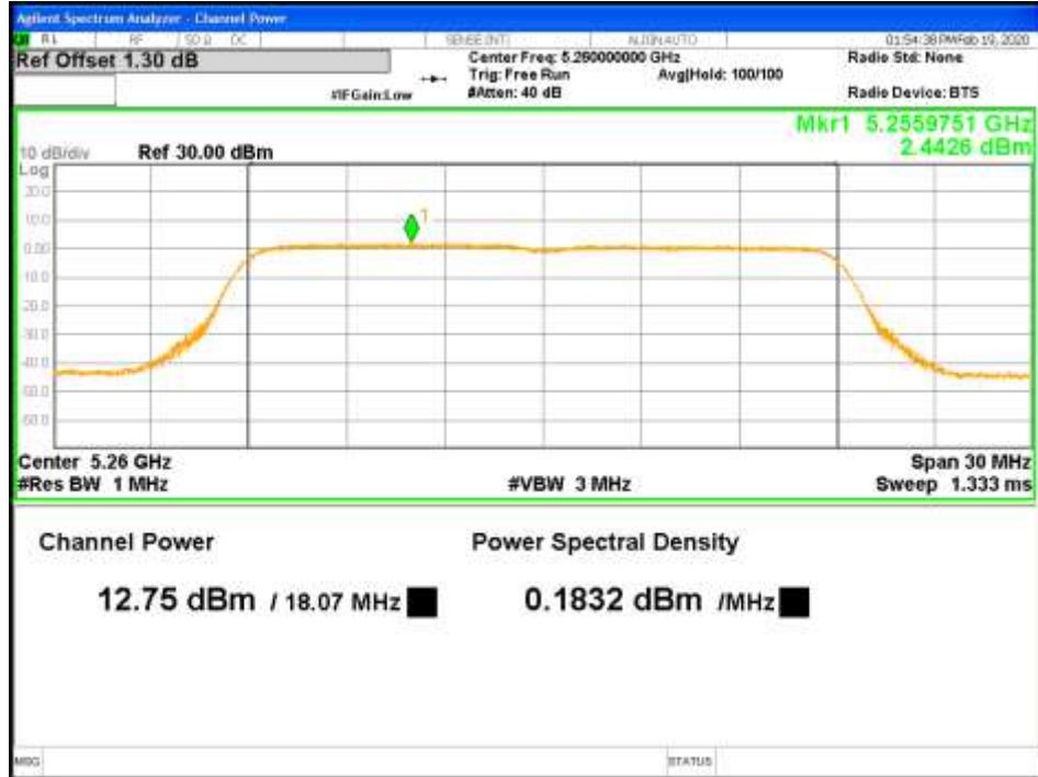
Figure 34: RMS Max Power-5260MHz-802.11ac VHT20-MCS0-TP13-2x2-CH1 (RSS)
