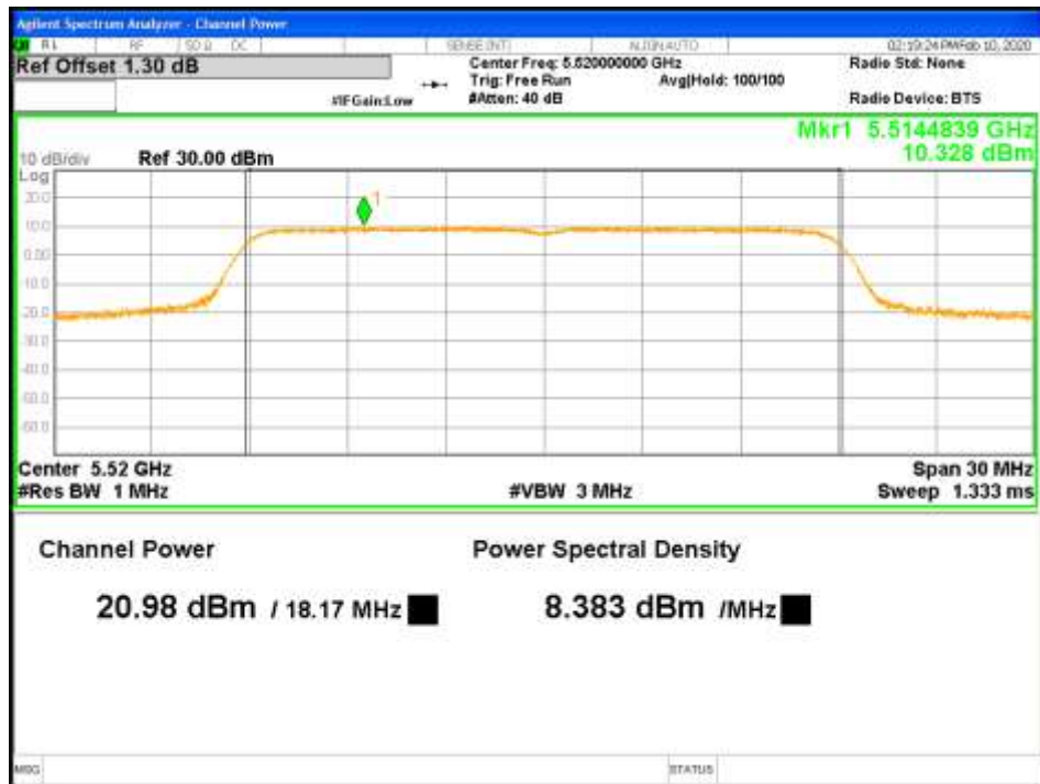
Figure 15: RMS Max Power-5520MHz-802.11ac VHT20-MCS0-TP21-1x2-CH0
