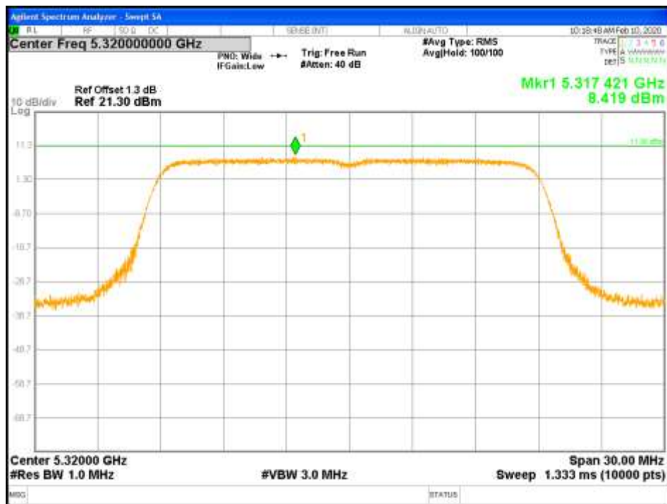
Figure 64: PPSD-5320MHz-802.11ac VHT20-MCS0-TP19-CH1-1x2 (RSS)
