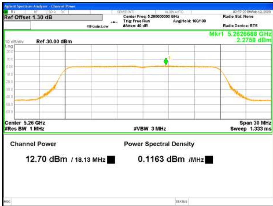
Figure 33: RMS Max Power-5260MHz-802.11ac VHT20-MCS0-TP13-2x2-CH0 (RSS)
