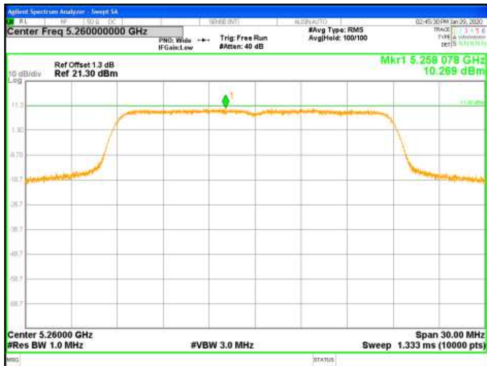
Figure 63: PPSD-5260MHz-802.11ac VHT20-MCS0-TP21-CH0-1x2 (FCC)
