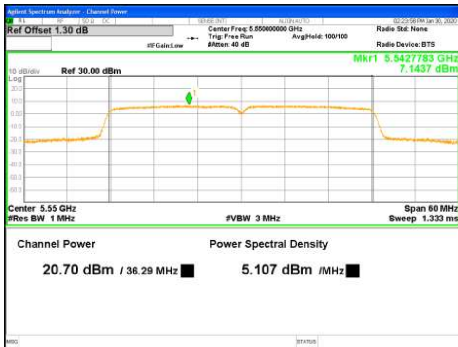
Figure 21: RMS Max Power-5550MHz-802.11ac VHT40-MCS0-TP21-1x2-CH0
