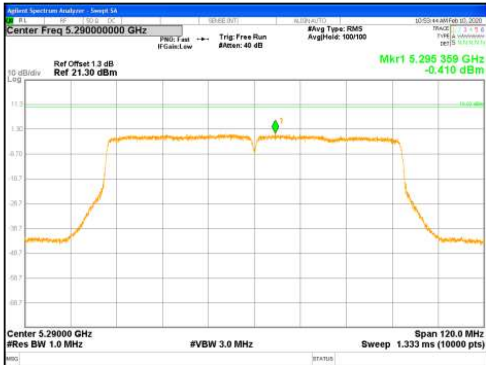
Figure 77: PPSD-5290MHz-802.11ac VHT80-MCS0-TP17-CH0-2x2 (FCC)
