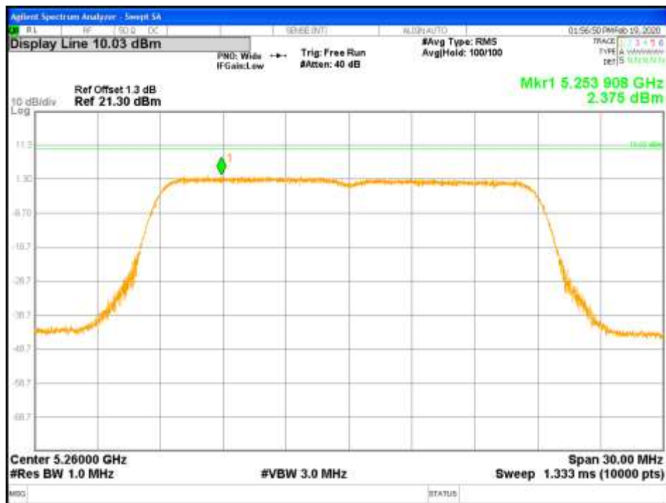
Figure 72: PPSD-5260MHz-802.11ac VHT20-MCS0-TP13-CH1-2x2 (RSS)
