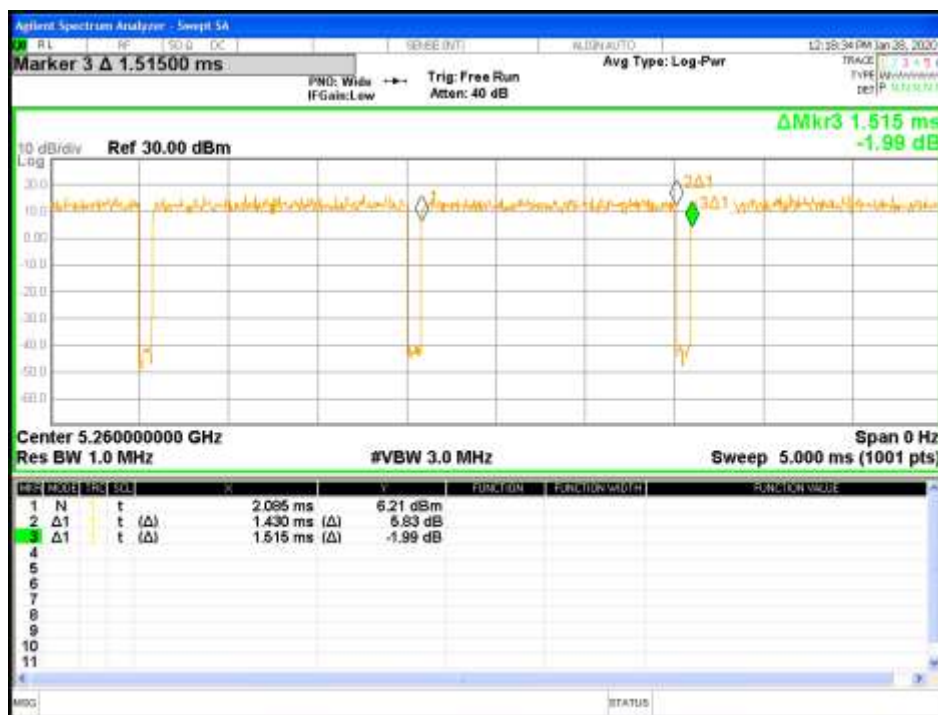
Figure 1: Duty Cycle for 802.11a at 5260MHz
