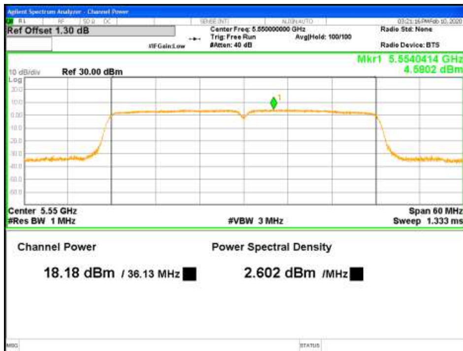
Figure 41: RMS Max Power-5550MHz-802.11ac VHT40-MCS0-TP18.5-2x2-CH0
