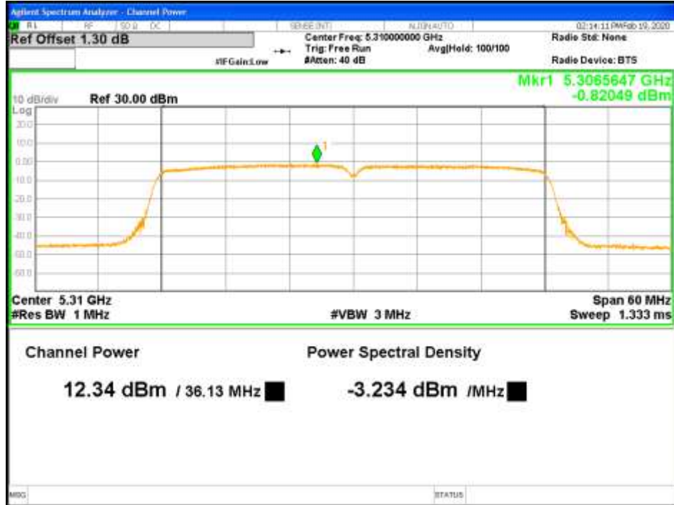
Figure 40: RMS Max Power-5310MHz-802.11ac VHT40-MCS0-TP13-2x2-CH1 (RSS)
