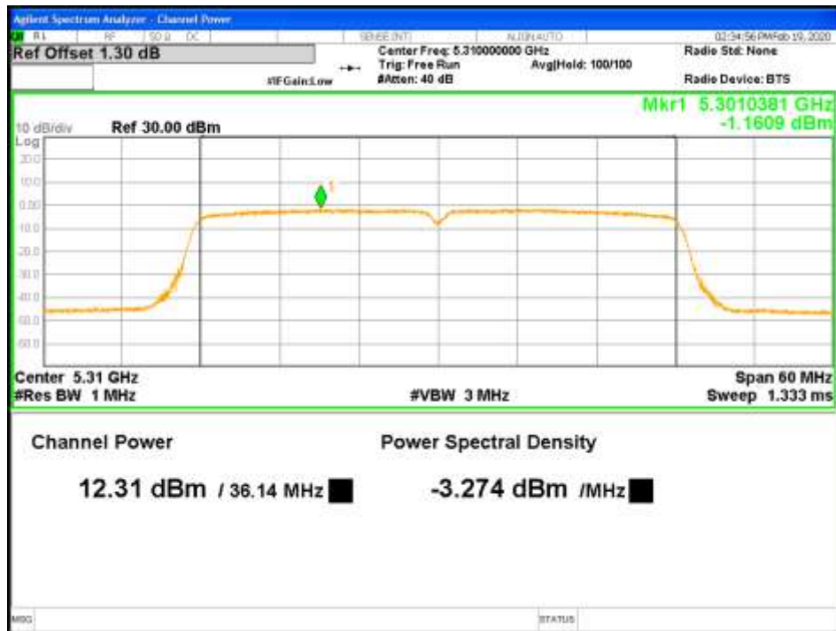
Figure 39: RMS Max Power-5310MHz-802.11ac VHT40-MCS0-TP13-2x2-CH0 (RSS)
