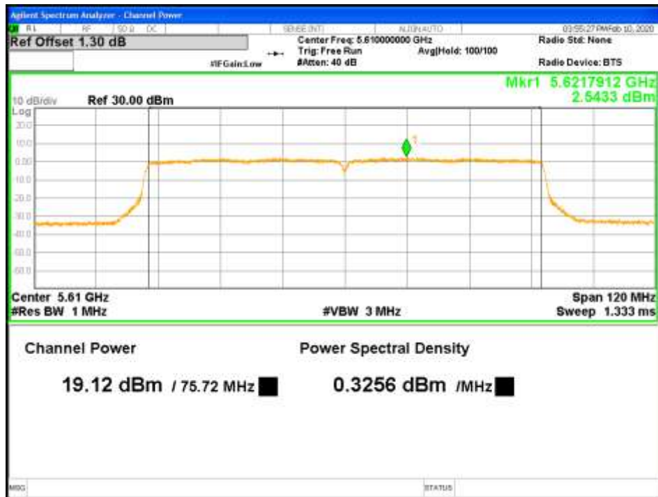
Figure 25: RMS Max Power-5610MHz-802.11ac VHT80-MCS0-TP20.5-1x2-CH0
