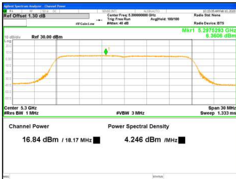
Figure 32: RMS Max Power-5300MHz-802.11ac VHT20-MCS0-TP17-2x2-CH1 (FCC)
