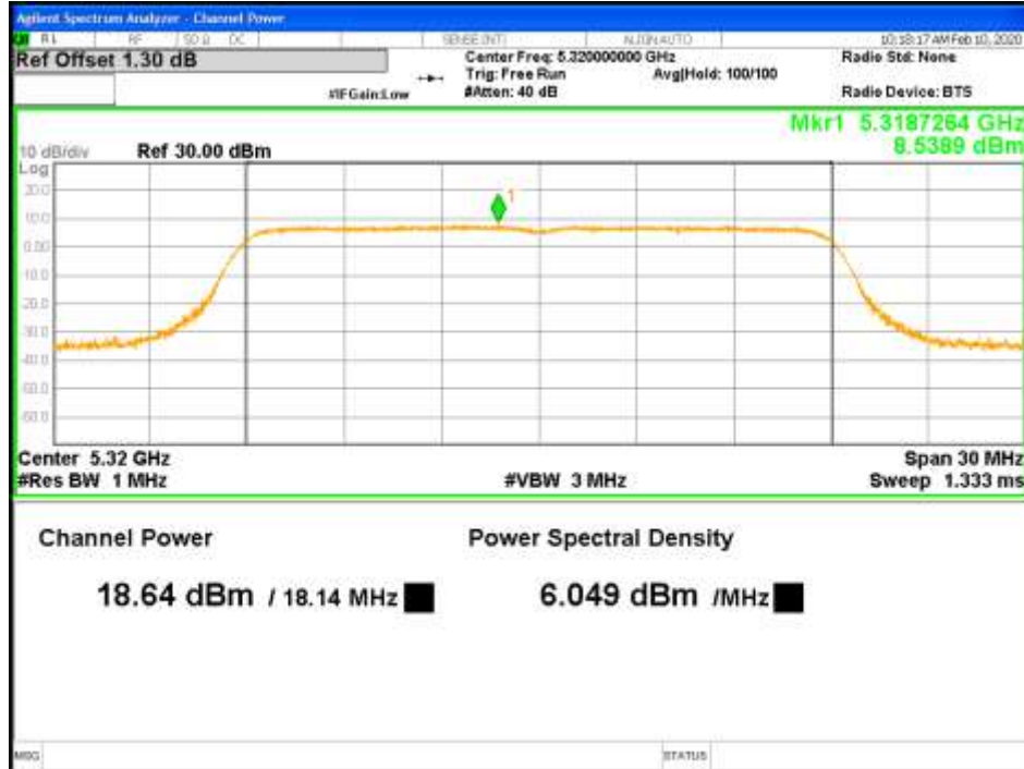
Figure 14: RMS Max Power-5320MHz-802.11ac VHT20-MCS0-TP19-1x2-CH1 (RSS)
