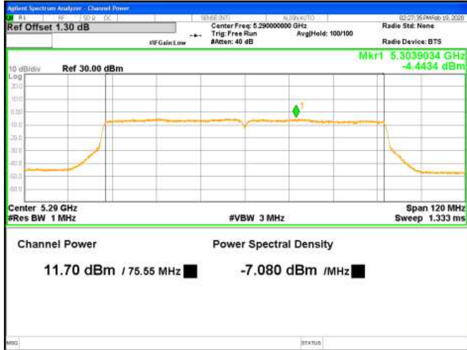
Figure 46: RMS Max Power-5290MHz-802.11ac VHT80-MCS0-TP13-2x2-CH1 (RSS)
