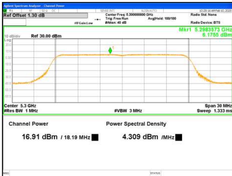
Figure 31: RMS Max Power-5300MHz-802.11ac VHT20-MCS0-TP17-2x2-CH0 (FCC)
