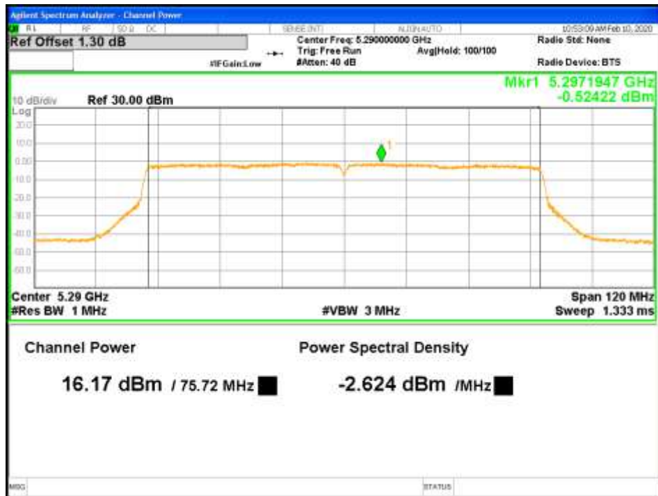
Figure 43: RMS Max Power-5290MHz-802.11ac VHT80-MCS0-TP17-2x2-CH0 (FCC)
