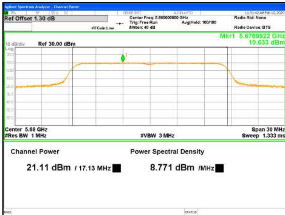
Figure 10: RMS Max Power-5680MHz-802.11a-6Mbps-TP21-1x2-CH1
