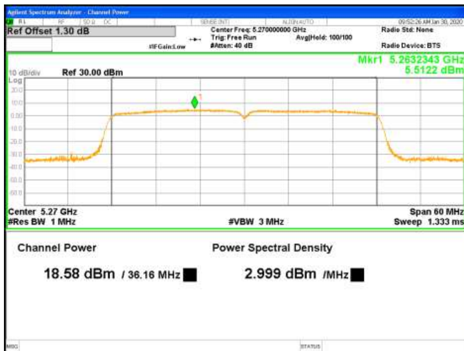
Figure 38: RMS Max Power-5270MHz-802.11ac VHT40-MCS0-TP18.5-2x2-CH1 (FCC)
