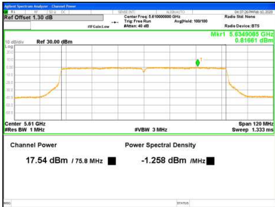
Figure 47: RMS Max Power-5610MHz-802.11ac VHT80-MCS0-TP19-2x2-CH0
