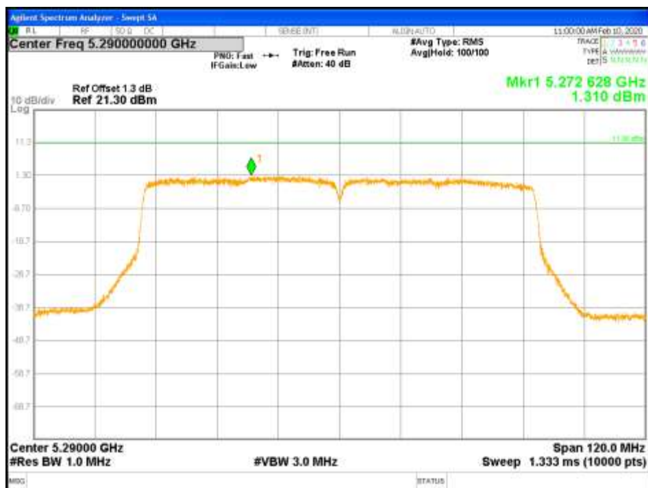
Figure 69: PPSD-5290MHz-802.11ac VHT80-MCS0-TP18.5-CH1-1x2 (FCC & RSS)
