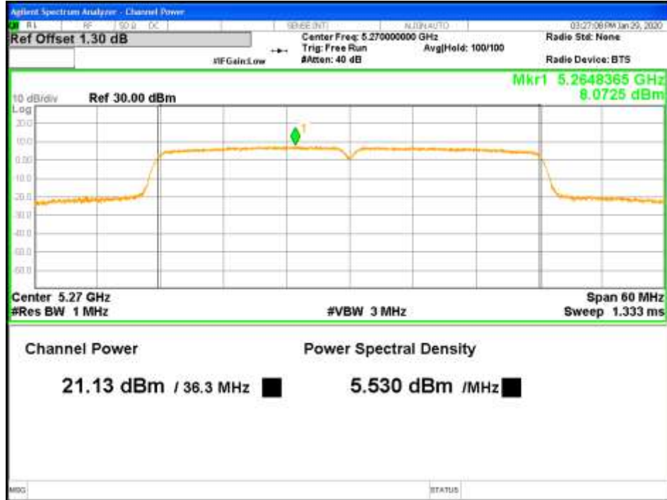
Figure 18: RMS Max Power-5270MHz-802.11ac VHT40-MCS0-TP21-1x2-CH1 (FCC)
