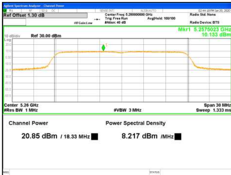
Figure 11: RMS Max Power-5260MHz-802.11ac VHT20-MCS0-TP21-1x2-CH0 (FCC)
