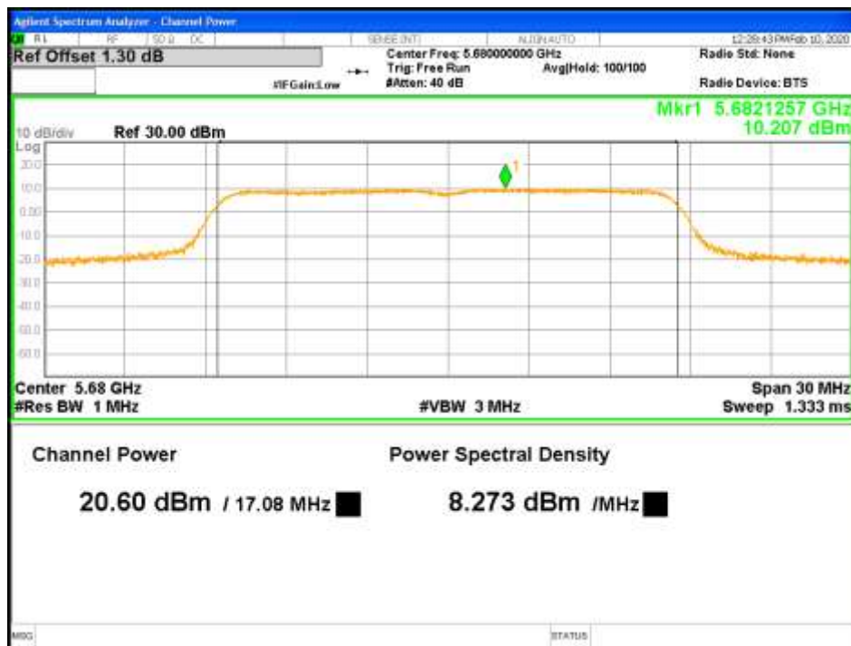
Figure 9: RMS Max Power-5680MHz-802.11a-6Mbps-TP21-1x2-CH0
