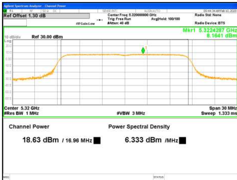
Figure 7: RMS Max Power-5320MHz-802.11a-6Mbps-TP19-1x2-CH0 (RSS)
