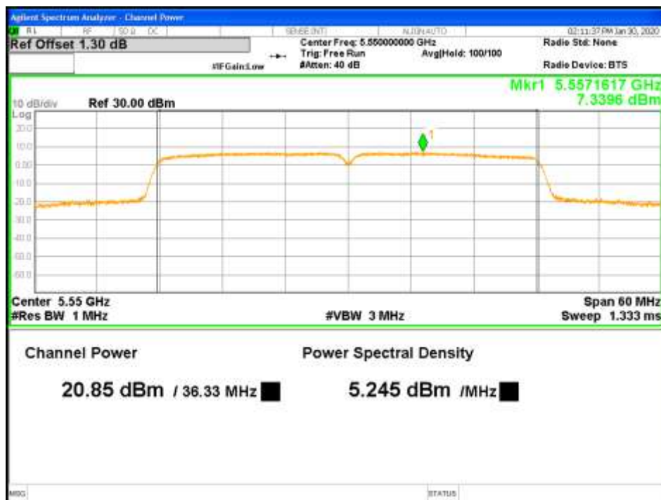
Figure 22: RMS Max Power-5550MHz-802.11ac VHT40-MCS0-TP21-1x2-CH1
