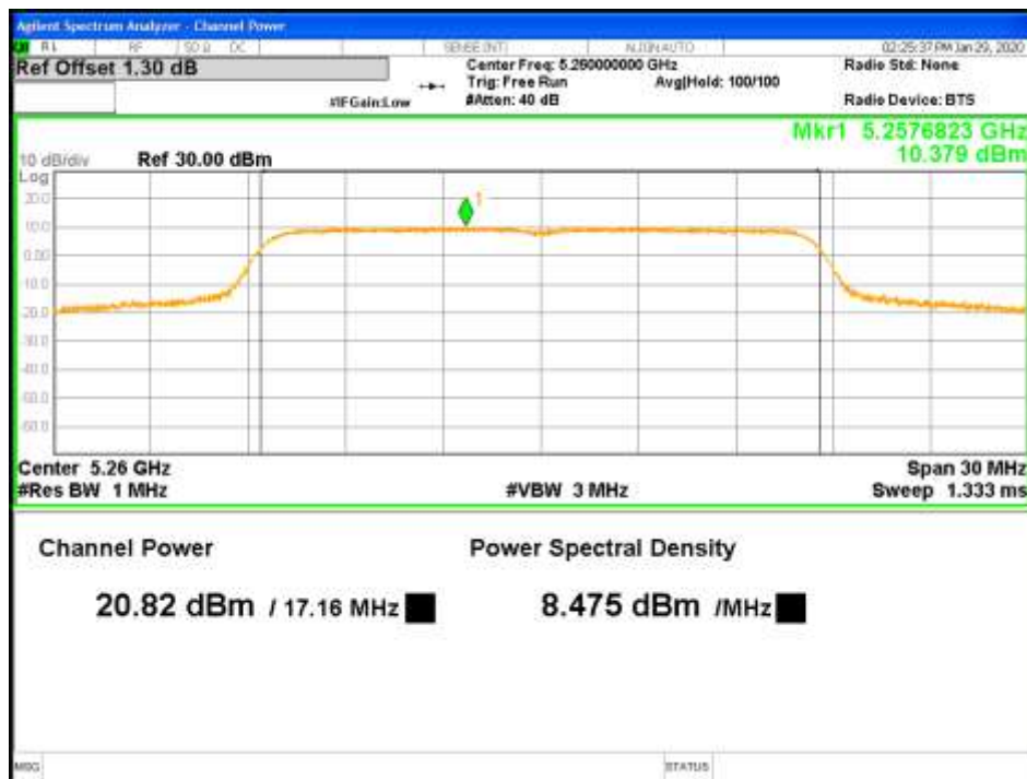
Figure 5: RMS Max Power-5260MHz-802.11a-6Mbps-TP21-1x2-CH0 (FCC)
