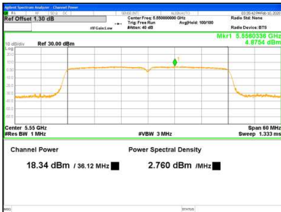
Figure 42: RMS Max Power-5550MHz-802.11ac VHT40-MCS0-TP18.5-2x2-CH1
