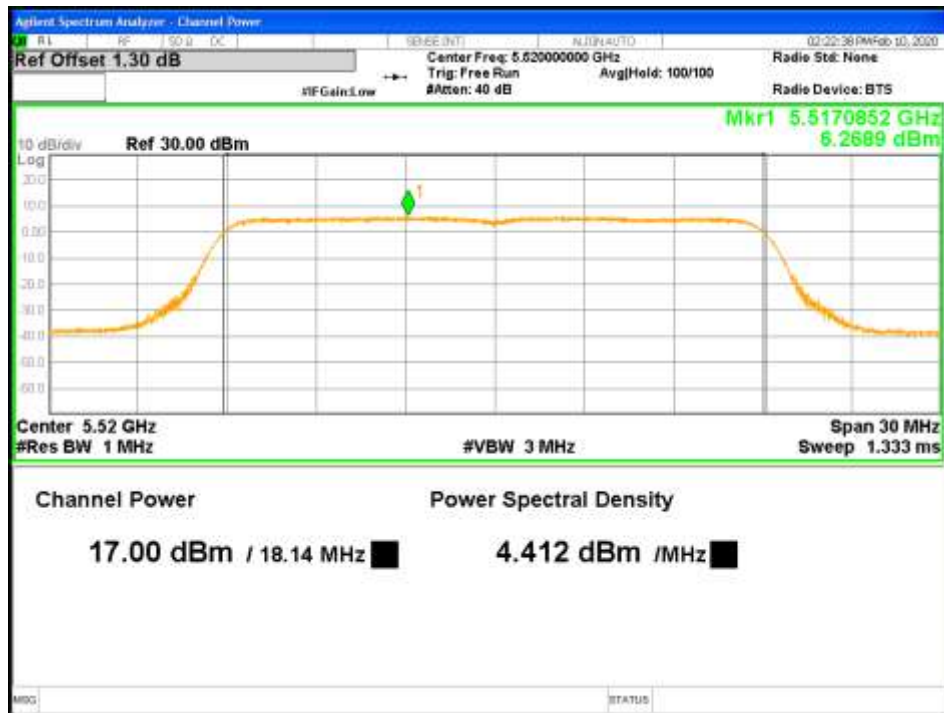
Figure 35: RMS Max Power-5520MHz-802.11ac VHT20-MCS0-TP17-2x2-CH0
