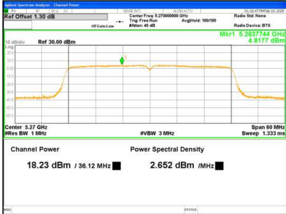
Figure 20: RMS Max Power-5270MHz-802.11ac VHT40-MCS0-TP18-1x2-CH1 (RSS)
