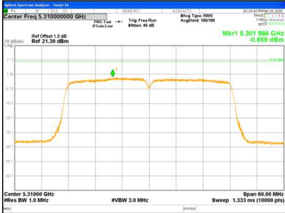
Figure 75: PPSD-5310MHz-802.11ac VHT40-MCS0-TP13-CH1-2x2 (RSS)
