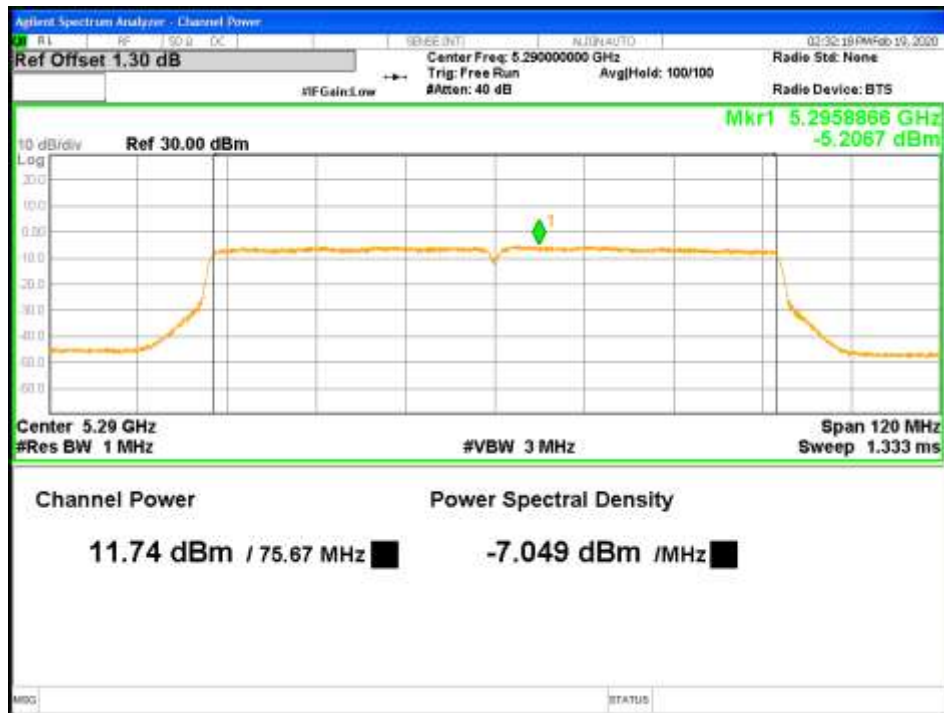
Figure 45: RMS Max Power-5290MHz-802.11ac VHT80-MCS0-TP13-2x2-CH0 (RSS)
