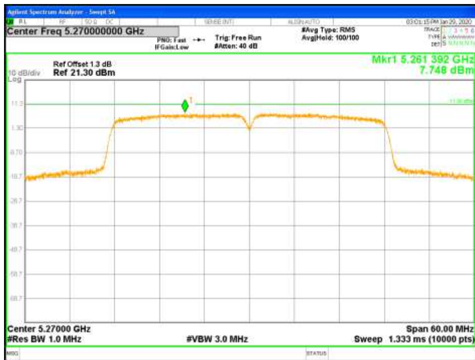
Figure 66: PPSD-5270MHz-802.11ac VHT40-MCS0-TP21-CH0-1x2 (FCC)
