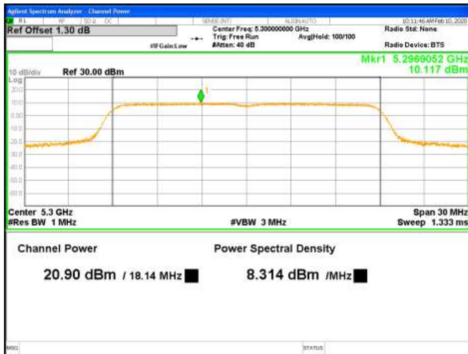
Figure 12: RMS Max Power-5300MHz-802.11ac VHT20-MCS0-TP21-1x2-CH1 (FCC)
