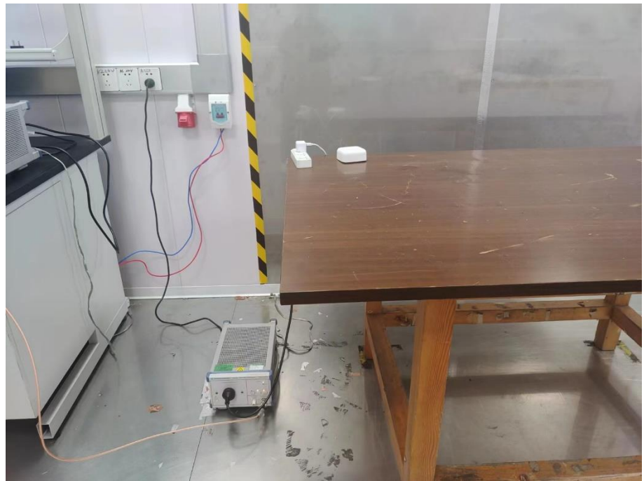
Conducted Emission Test Setup
