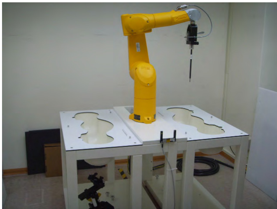
Fig.1 Photograph of the SAR measurement system
