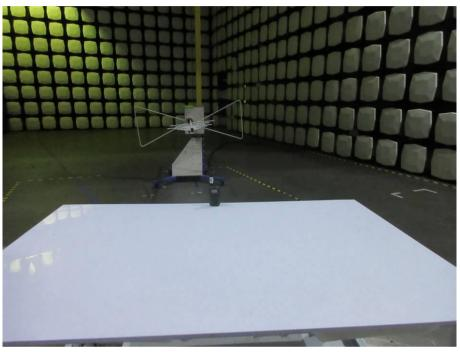
Radiated Emissions (Above 1GHz) Test Setup
