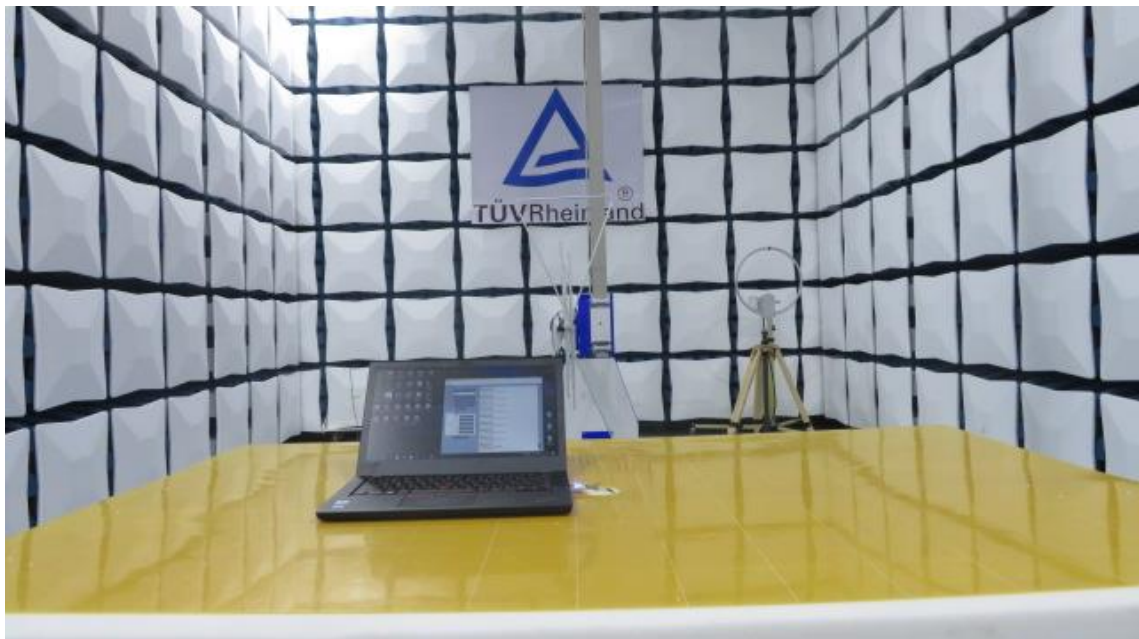
Photograph 2: Set-up for Spurious Emissions (1GHz-18GHz)
