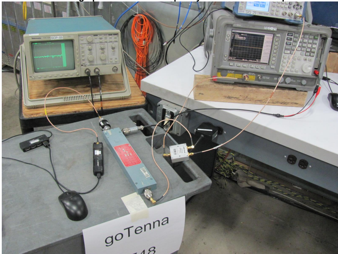
Photograph of Transient Frequency Behavior Test Setup
