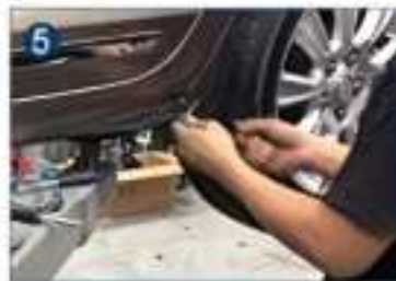
5. Use the zip tie to tie up the extra cable and hide it.
