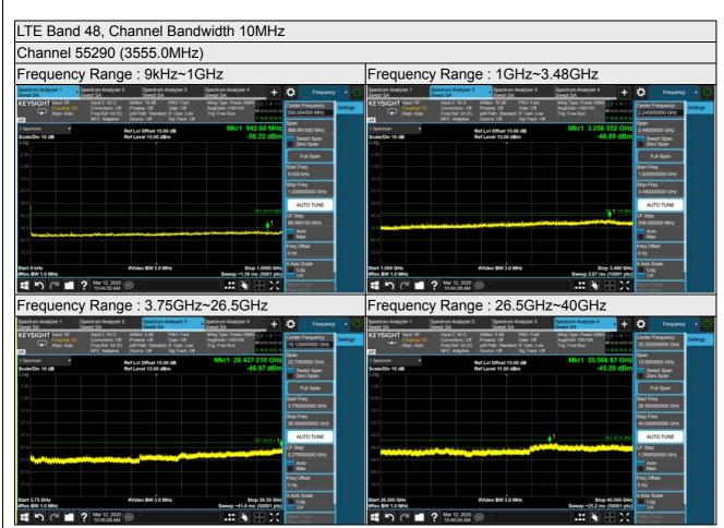
Note: The signal at 9 kHz is IF signal from spectrum analyzer.
