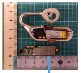
Remove RF shield of the PCB
