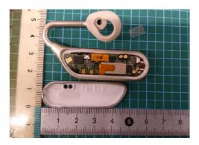
Remove PCB (below RED box is the antenna location for bluetooth)
