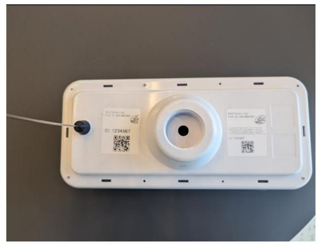
Label with **FCC ID: 2ALN6GWA** will be located at the side of the sensor. The statement according to FCC part 15 §15.19(a)(3) is placed in User's Manual, page 12.
