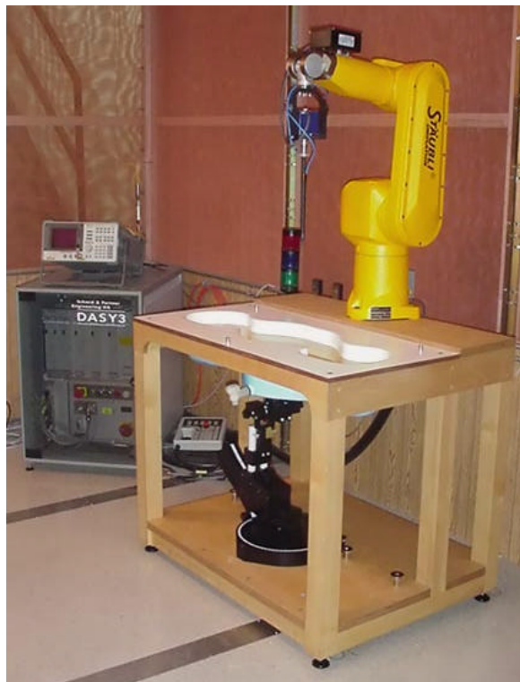
DASY3 SAR Measurement System
