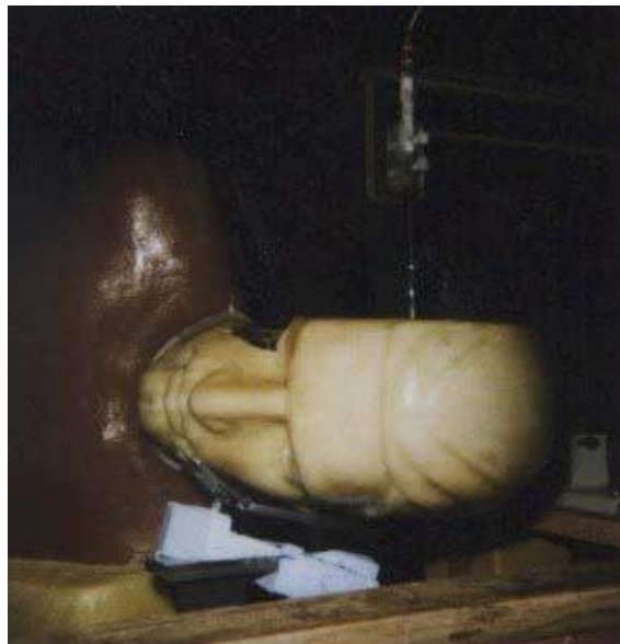
Fig. b. The Telson Model TDC 8020 Wireless Telephone held against the phantom model used for measurement of the SAR distribution. For clarity the front edge of the Styrofoam holder is removed.
