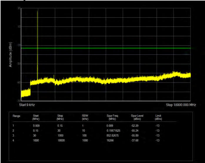
Band4 QPSK BW=5MHz Channel=20375 RB Size=1 Position=#0
