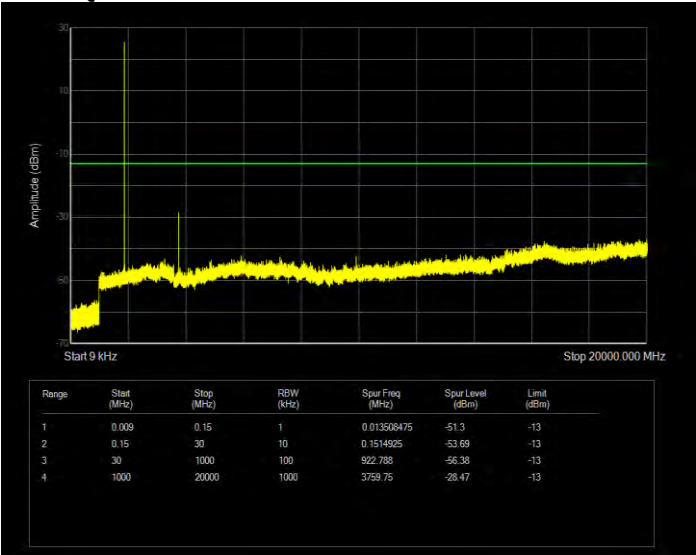
Band2 16QAM BW=1.4MHz Channel=19193 RB Size=1 Position=#0
