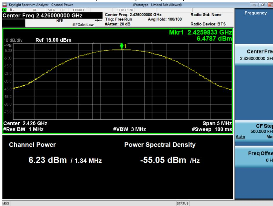
**Maximum Transmit Power, 2480 MHz, GFSK, 1 Mbps**
