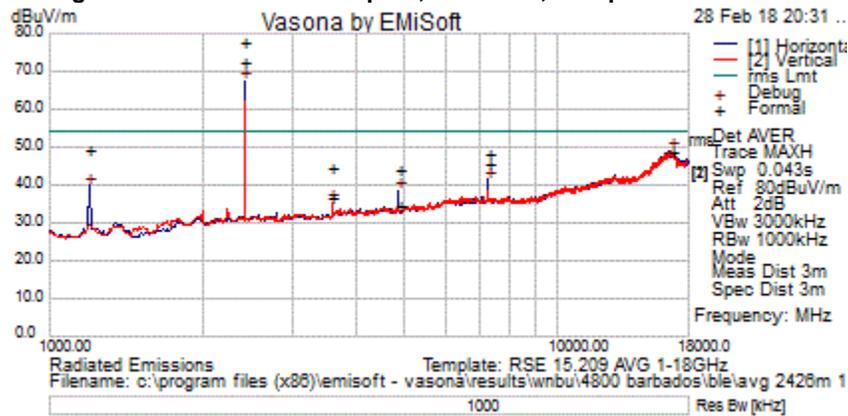
**Average Radiated Transmitter Spurs, 2480 MHz, 1 Mbps GFSK**
