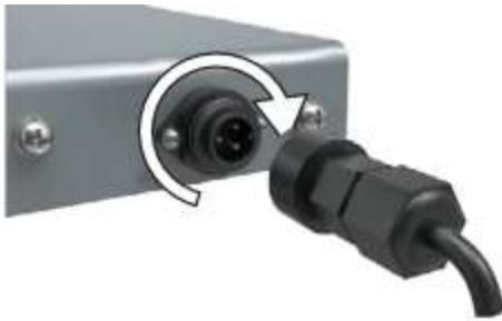
Figure 15. Connect Power Cable at Rear Side
