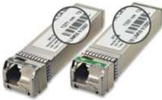
Figure 3. Single Port SFP Module
