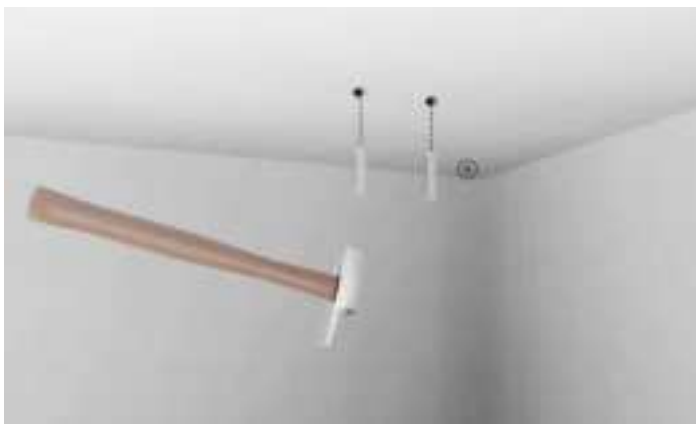
Figure 50. Insert Plastic Wall Plugs
