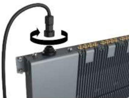
Figure 20. Connect power cable at the rear of the unit
