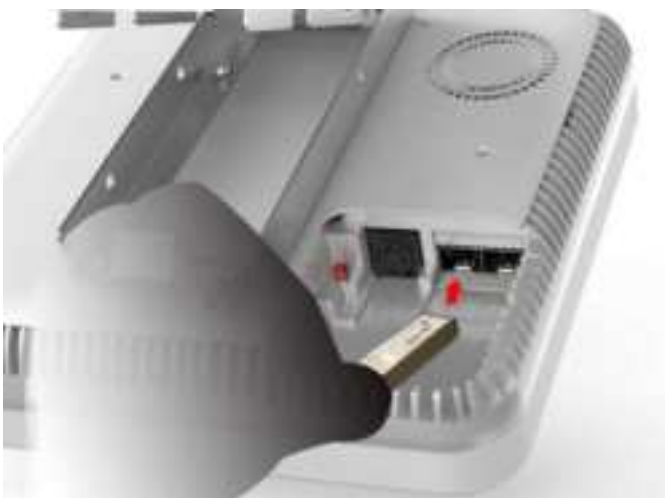
Figure 73. SFP Module Insertion
