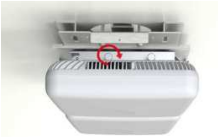
Figure 77. Tighten the Screws
