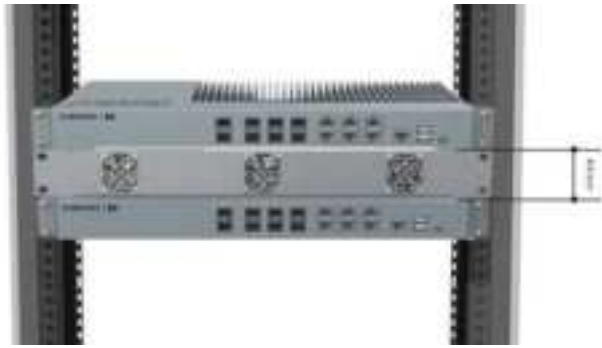
Figure 27. Separation of Adjacent EU-O
