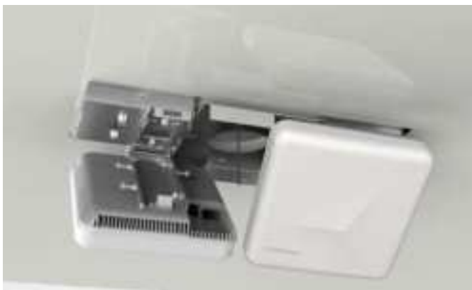
Figure 72. Buckle the Bracket 2
