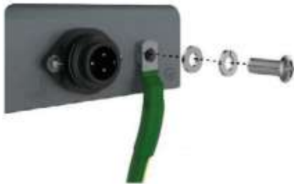
Figure 29. Connect Ground Cable at Rear Side
