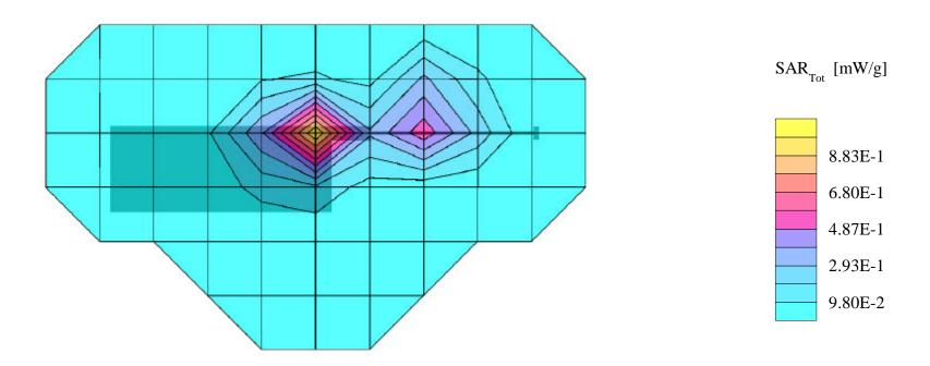
Generic Twin Phantom; Flat Section; Probe: ET3DV5 - SN1370 -- Probe Cal Date 02/00 Med. Parameters 1900 MHz Muscle:  $\sigma$  = 1.85 mho/m  $\epsilon_r$  = 54.2  $\rho$  = 1.00 g/cm³; Antenna Position -- In; Crest Factor 1.0 SAR (1g): 0.933 mW/g, SAR (10g): 0.530 mW/g
