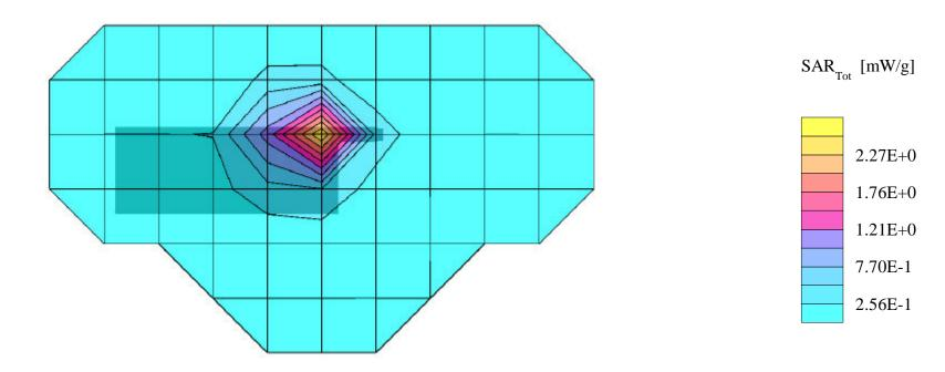
Generic Twin Phantom; Flat Section; Probe: ET3DV5 - SN1370 -- Probe Cal Date 02/00 Med. Parameters 1900 MHz Muscle:  $\sigma$  = 1.85 mho/m  $\epsilon_r$  = 54.2  $\rho$  = 1.00 g/cm³; Antenna Position -- Out; Crest Factor 1.0 SAR (1g): 1.13 mW/g, SAR (10g): 0.604 mW/g
