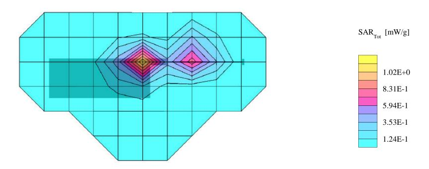
Generic Twin Phantom; Flat Section; Probe: ET3DV5 - SN1370 -- Probe Cal Date 02/00 Med. Parameters 1900 MHz Muscle:  $\sigma$  = 1.85 mho/m  $\epsilon_r$  = 54.2  $\rho$  = 1.00 g/cm³; Antenna Position -- In; Crest Factor 1.0 SAR (1g): 0.989 mW/g, SAR (10g): 0.555 mW/g
