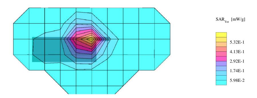
Generic Twin Phantom; Flat Section; Probe: ET3DV5 - SN1370 -- Probe Cal Date 02/00 Med. Parameters 1900 MHz Muscle:  $\sigma$  = 1.85 mho/m  $\epsilon_r$  = 54.2  $\rho$  = 1.00 g/cm³; Antenna Position -- Out; Crest Factor 1.0 SAR (1g): 1.21 mW/g, SAR (10g): 0.630 mW/g
