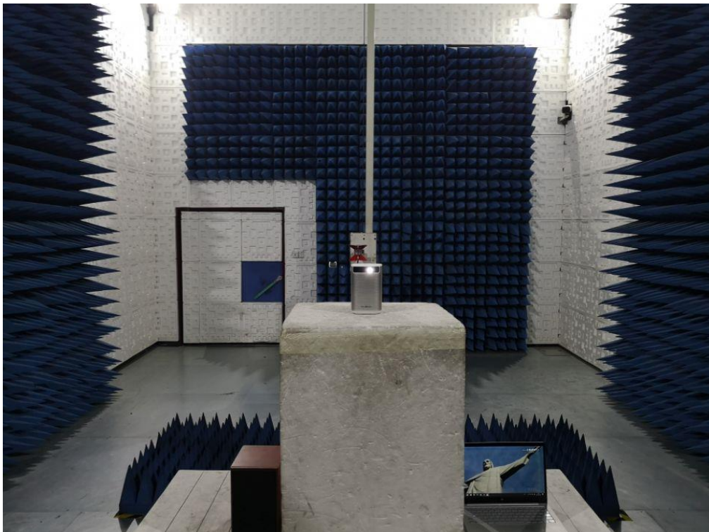
RADIATED EMISSION TEST SETUP ABOVE 1GHZ
