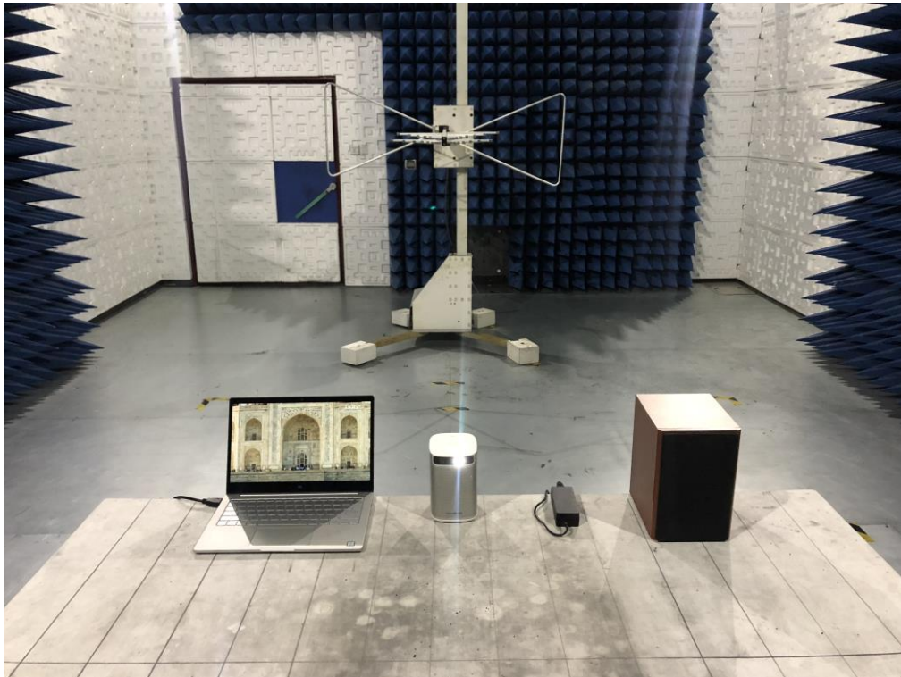
RADIATED EMISSION TEST SETUP ABOVE 1GHZ
