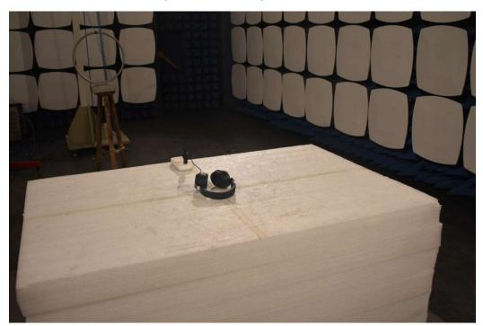
3. Radiated emission (9KHz-30MHz)
