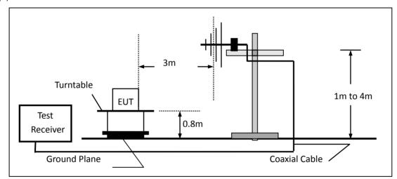
(c) For radiated emissions above 1000MHz
