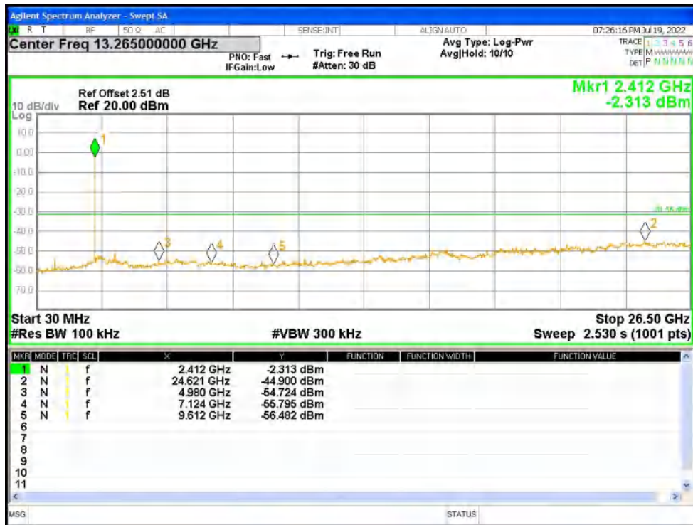
Tx. Spurious NVNT b 2437MHz Ant1 Ref
