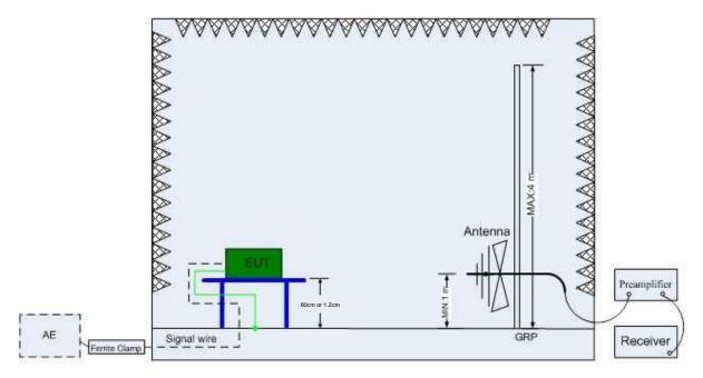
Radiated tests above 1GHz
