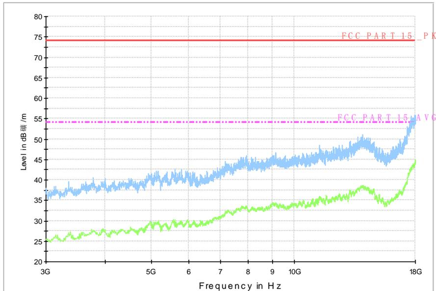
Fig.11. Radiated emission: Channel 78, 3 GHz - 18 GHz
