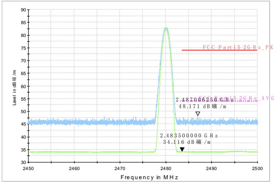
Fig.13. Radiated emission (Power): High Channel
