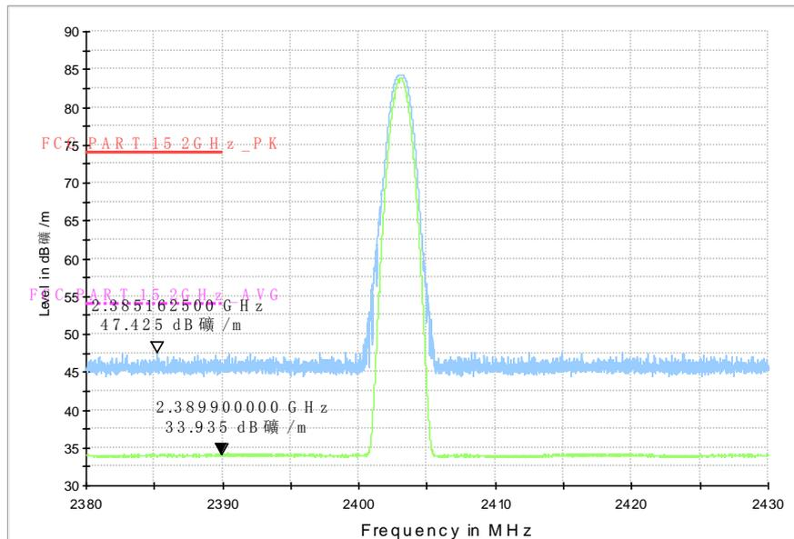
Fig.12. Radiated emission (Power): Low Channel
