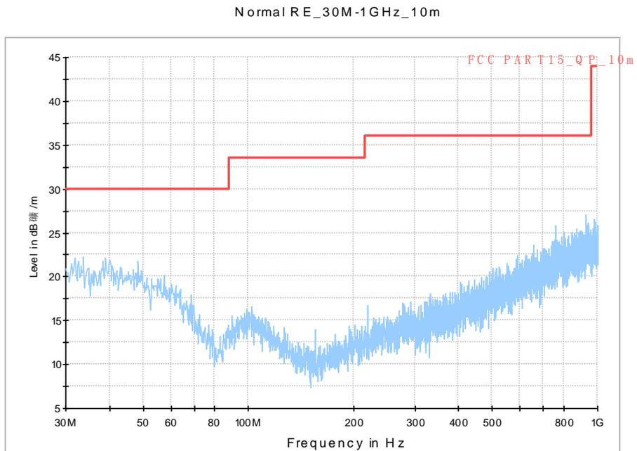
Fig.6. Radiated emission: Channel 39, 30 MHz - 1 GHz
