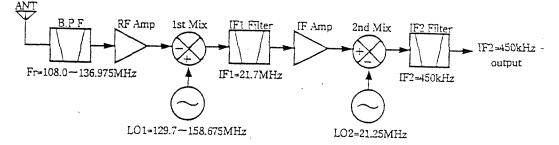
The first frequency converter circuit (1st Mixer) mixes the received signal with the first local oscillator signal, whose frequency (LO1) is higher than the selected receive frequency (Fr) by the first intermediate frequency (IF1 = 21.7 MHz), to down-convert the received signal to the first intermediate frequency band (Fr to IF1). Since LO1 is determined so that it is always higher than Fr by IF1 (21.7 MHz), Fr and LO1 has always the relation as expressed by the following equation:
