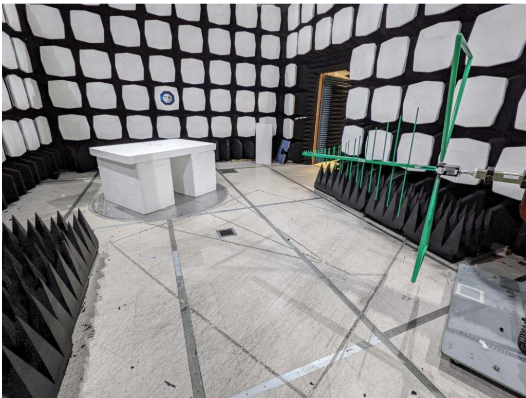
Figure 3: Equipment Under Test – Radiated Emissions <1GHz
